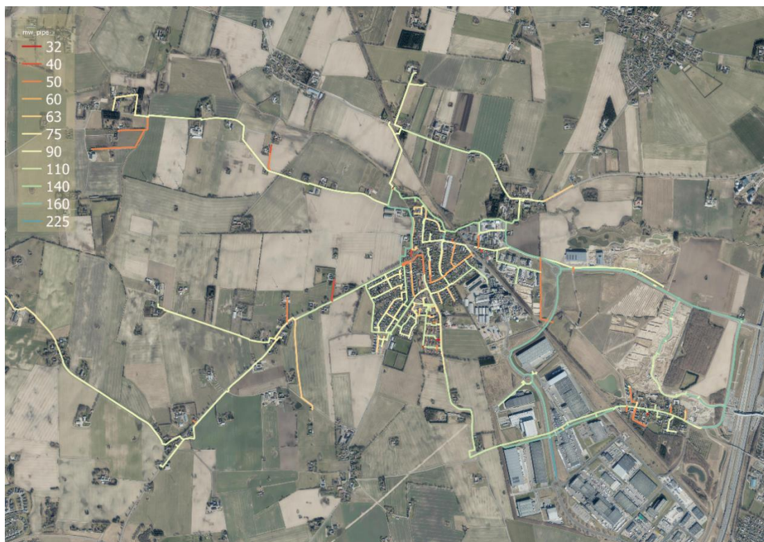
Figure 7. Overview of the different dimensions of the water distribution system.
