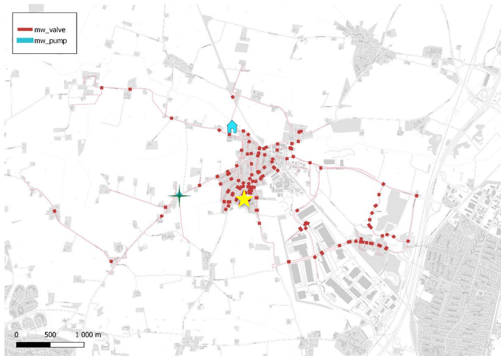
Figure 5. Overview of the water distribution system. Valves (red), waterworks (light blue), booster pump (green) and backup pump (yellow) are marked.
