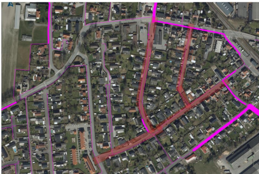
Figure 7777. Water utility of Lille Skensved's future plans in renovation of pipes marked in red. Criticality results of scenario 1 displayed in purple.
