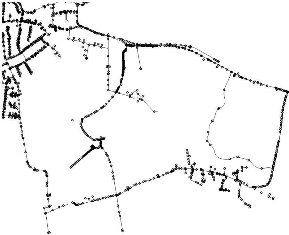
Figure 4. Polylines (pipes) and points (junctions) imported.
