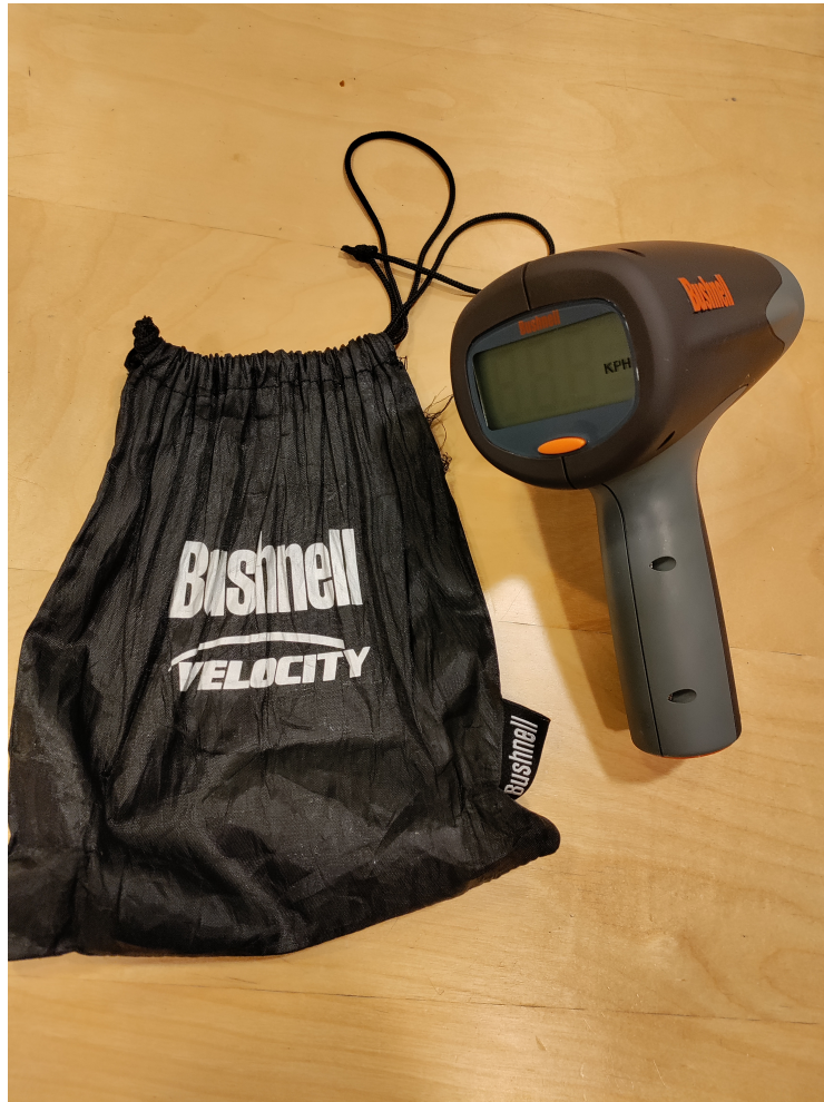
Figure 19: Velocity gun used to measure the Throwing velocity of the handball players' step shot.
