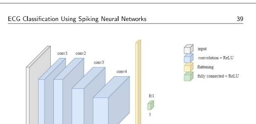
Figure 3.5: Our final NN structure with 114,453 trainable parameters.
