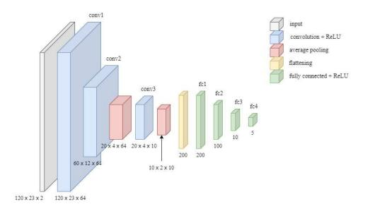
Figure 3.4: Structure of our NN with 105,279 trainable parameters.
