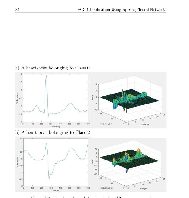
**Figure 3.3:** Two heart-beats belonging to two different classes and the real part of their STFT. The first one is a normal beat. The second one, which is a ventricular escape beat, has some distinguishing characteristics such as wide QRS complex and abnormal morphology of QRS complex.
