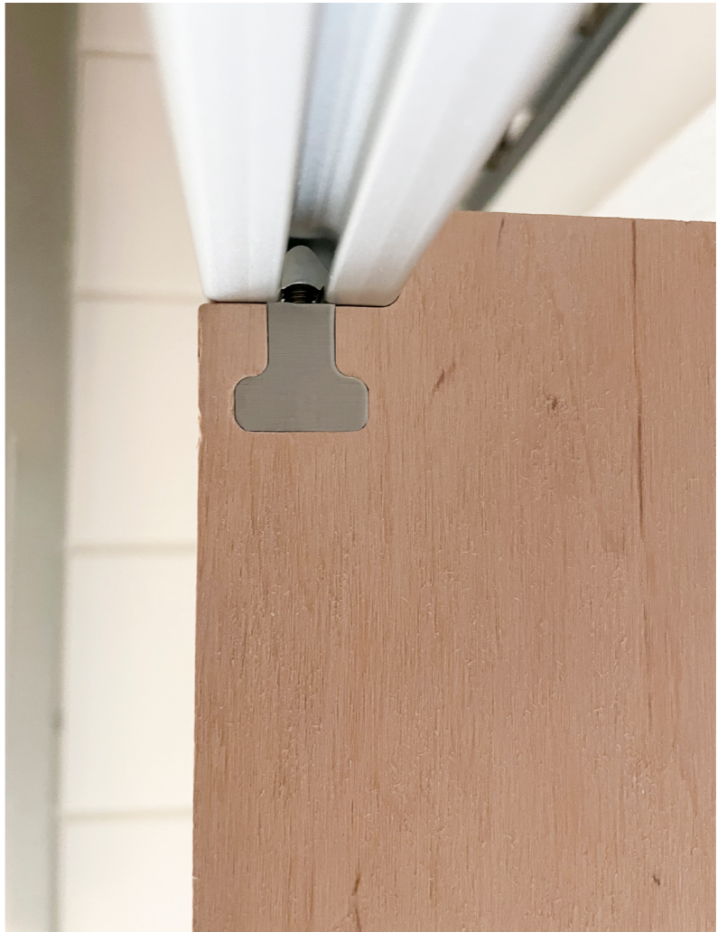
Proof of concept; decided on that profile we moved forward with trying out different connectors. In the picture above is the first well-working connector made. The structure was surprisingly stable, this was really a breakthrough, and the proof of concept needed to move even further with this profile.
