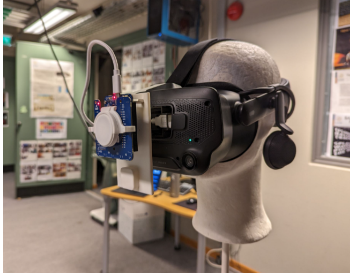
Figure 3.5: The finished VR prototype, with the XE121 PCR sensor connected through USB and 3D-printed parts to the attachment point of the VR headset
