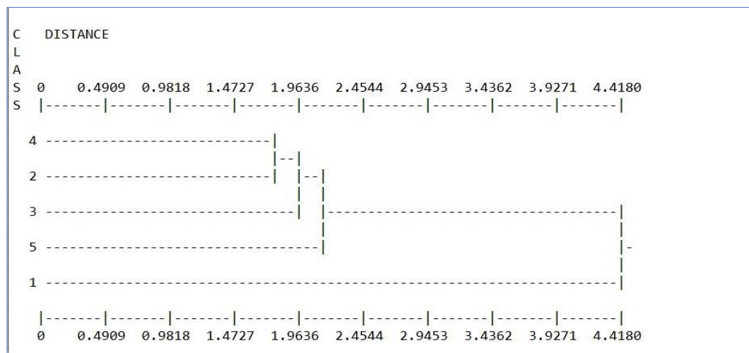
Figure 8: Dendrogram of classes created showing distance among values (1: vegetation, 2: soil/sparse vegetation, 3: tile roofs, 4: impervious surfaces, 5: archaeology/rock).
