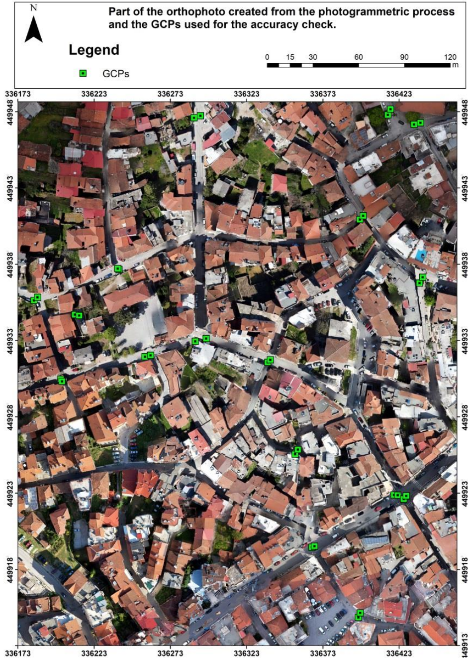
Figure 14: Part of the orthophoto resulted from the photogrammetric process from the UAV data using GCPs.
