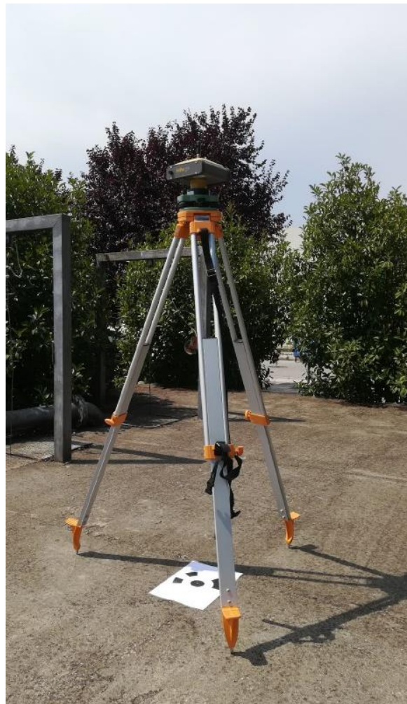
Figure 5: Example of a GCP measurement with GPS.
