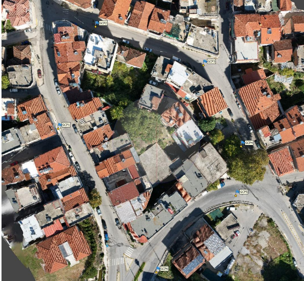
Figure 2: Distribution of GCPs in a part of the study area for a UAV image set.
