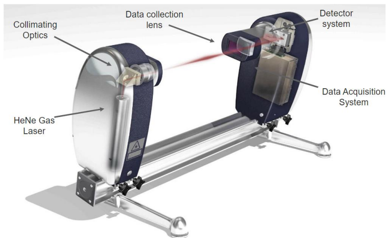
Figure 12. Presentation of the laser diffraction system with the different parts [13].
