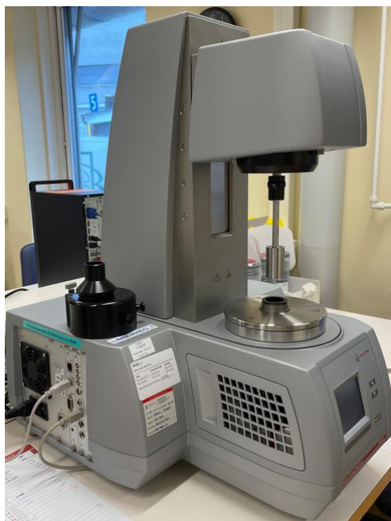
Figure 10. Anton Paar MCR 302 with double-gap geometry in use [picture taken on-site].
