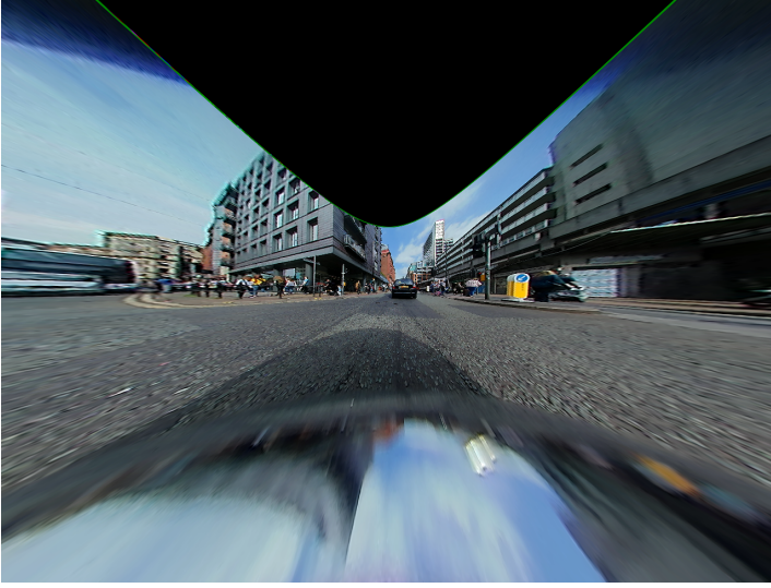
Figure 3.4 Zoomed-out version of the rectilinear projection. The image demonstrates the deviation from the true transformation in the 4th-order polynomial function as we get closer to the images edges.
