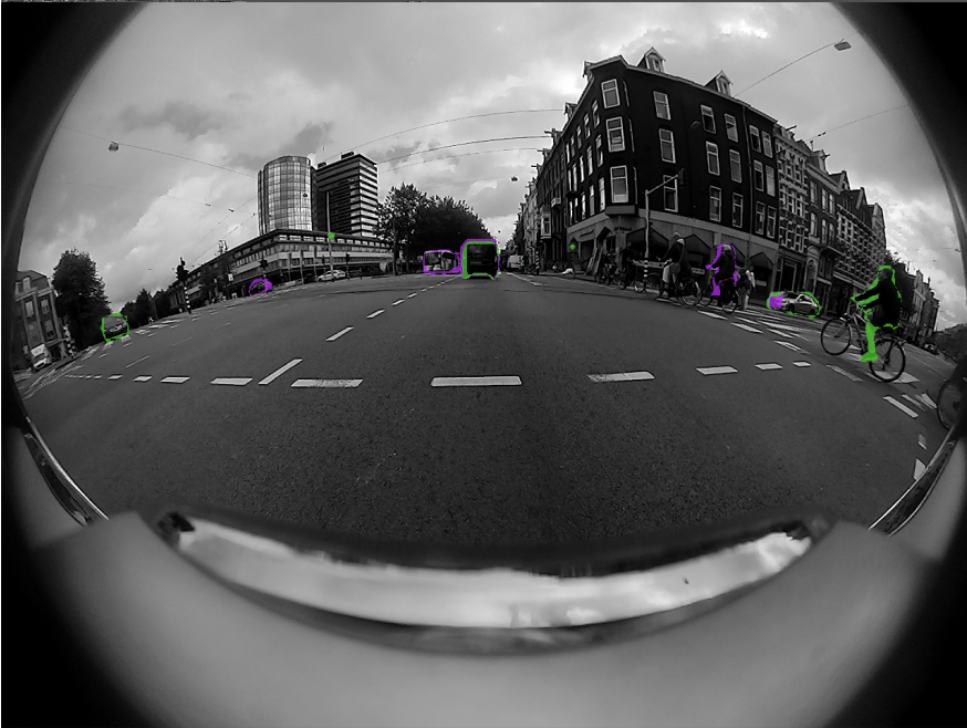
Figure 5.22 Areas marked in green show the false positive and false negative regions of the fisheye model's predictions. Areas marked in purple show the same for the rectilinear model, with predicted segmentations that have been mapped back to the fisheye distortion. There is no discernible difference in error between the two models that can be gathered from this image alone.
