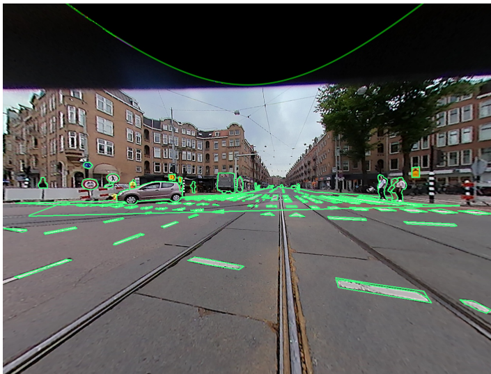
Figure 1.12 The rectilinear corrected image with the maximum number of objects for segmentation
