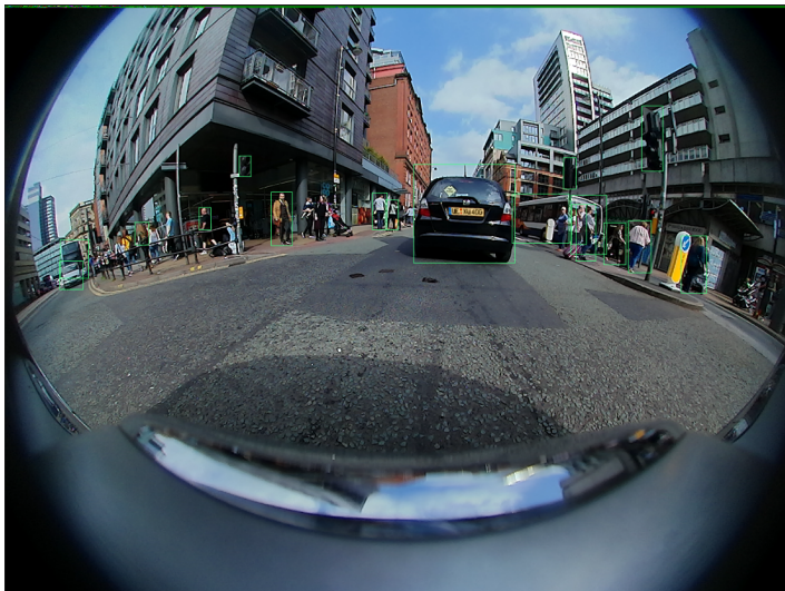
Figure 4.1 Example of an annotated fisheye image with 2D bounding boxes, taken directly from the WoodScape dataset.
