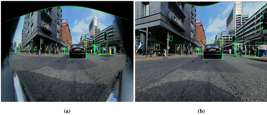
Figure 4.4 Example of a cylindrical and a rectilinear image with the final bounding box annotations
