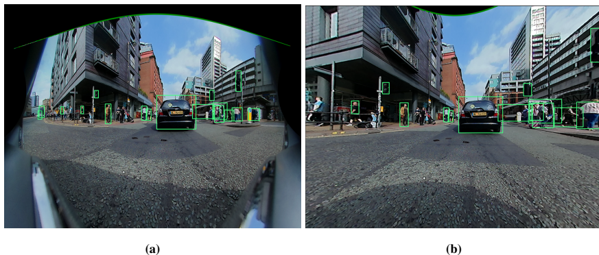
Figure 4.2 Example of a cylindrical and a rectilinear image with the resulted bounding box coordinates after applying the projection considering two coordinates of the bounding boxes from the fisheye image. Notice the objects being cropped by the resultant bounding box, particularly in objects near the edge of the image in the rectilinear projection.
