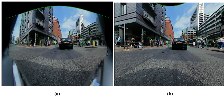
Figure 4.3 Example of a cylindrical and a rectilinear image with the remapped bounding box coordinates after applying the projection considering four coordinates of the bounding boxes from the fisheye image. The resulting skew of the bounding box should be corrected in order to work better with the YOLO object detector (see figure 4.4).
