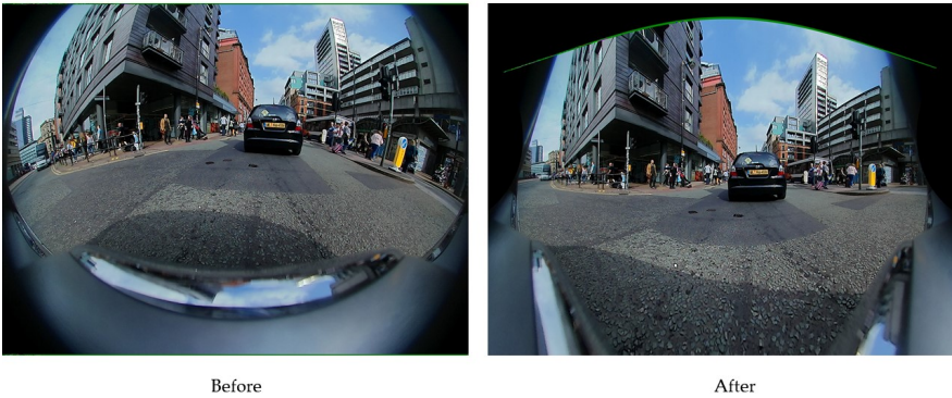
Figure 3.1 Before and after of a cylindrical projection. The vertical axis has clearly been undistorted, evidenced by the straightness in the height of all the buildings. The horizontal axis remains slightly distorted. This type of projection is helpful for maintaining the horizontal field of view while mitigating any vertical distortion.
