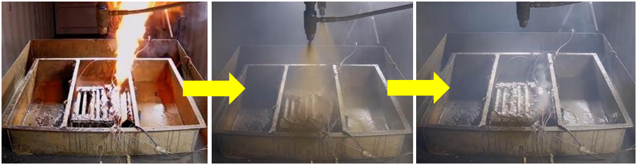
Figure 16 Demonstration of AVD encapsulates LIB cells to extinguish the fire and stop propagation [53].
