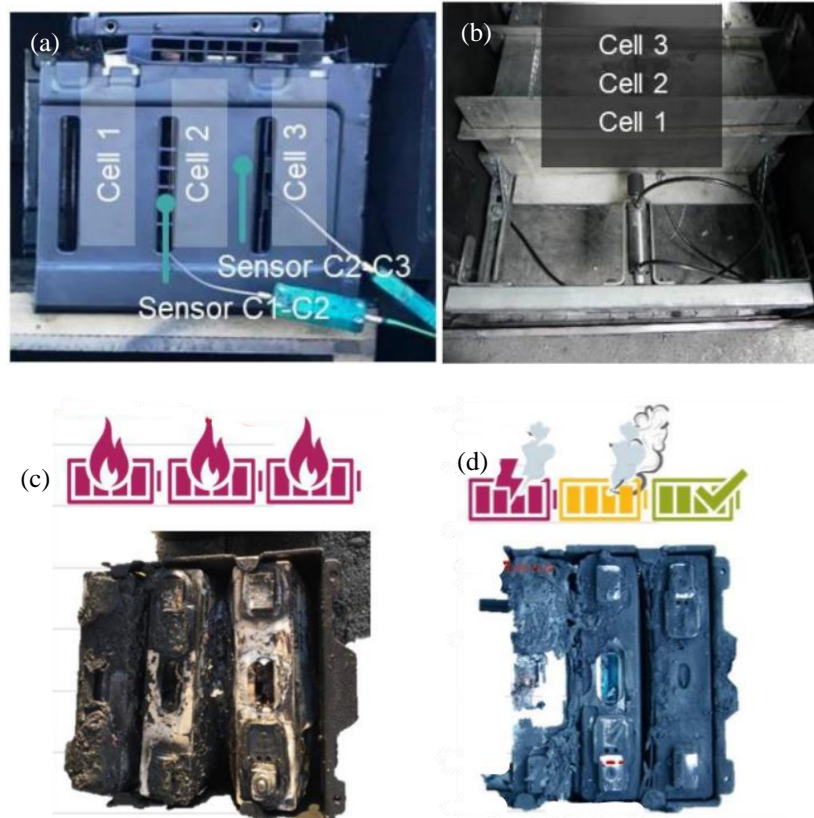
Figure 25 (a) Battery module; (b) Battery module in N 2 chamber; (c) Aftermath @ 20.9% O 2 concentration; and (d) Aftermath @ 11.3% O 2 concentration [50].
