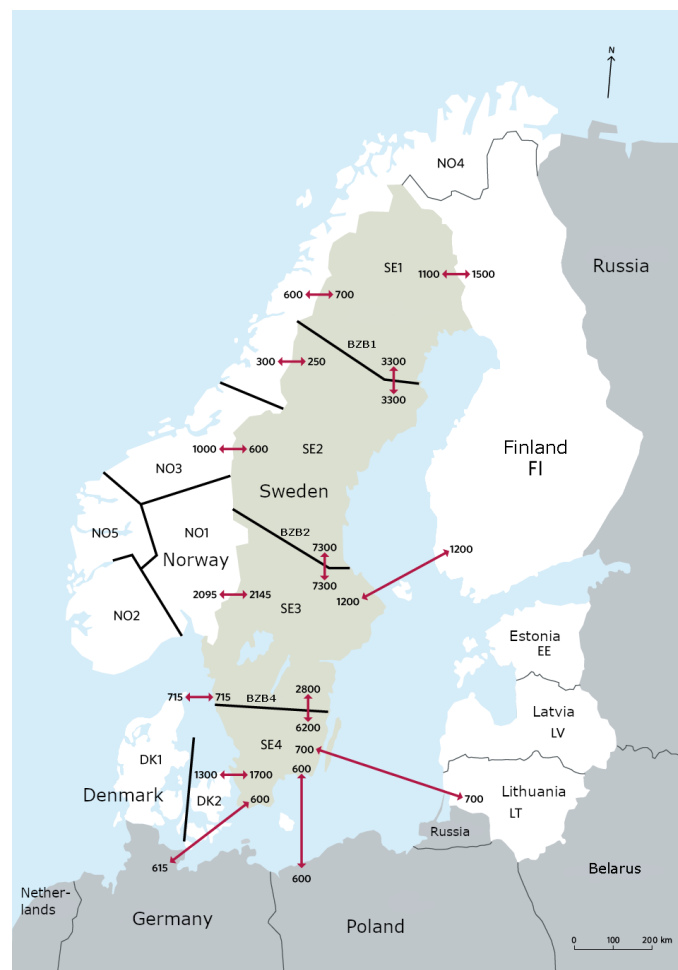
Figure 3: NTC transmission capacities within, to and from Sweden in 2022. Translated version of figure from SvK [11].
