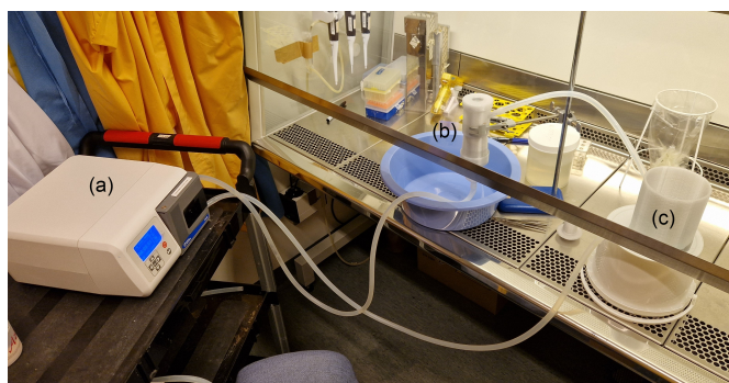
Fig. 5. Setup of the entire testing environment. Key elements shown are the peristaltic pump (a), the valve holder section and compliance chamber (b) and the fluid reservoir (c).
