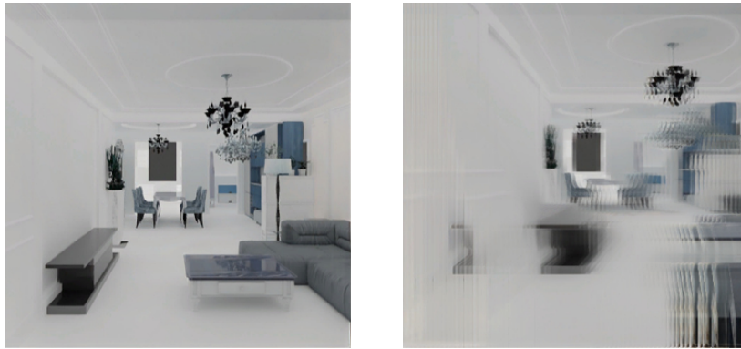
Figure 2.4: Example of the "stack-of-cards effect" caused by rendering from a baseline that is too large.
