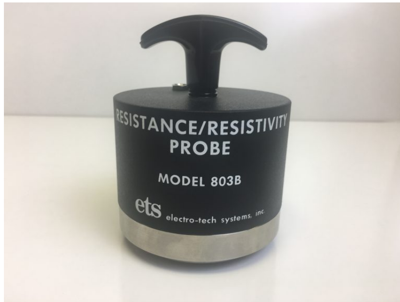
Figure 11: Image of probe used to measure surface and volume resistivity. The probe is placed on the sample using a 100 V bias to measure surface resistivity and 10 V bias for volume resistivity.
