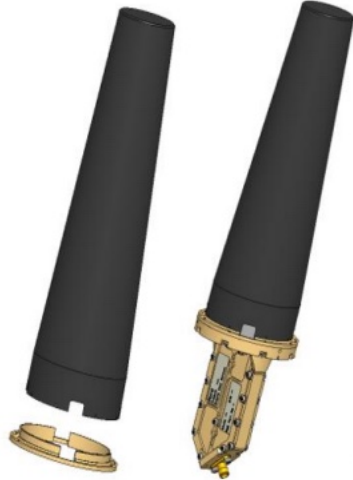
Figure 1: Depiction of Beyond Gravity’s Ultem 2300 radomes. Hollow cone-shaped radome with applied black surface coating. The aluminum chassis is shown as yellow in the image, is connected with the radome. To provide a grounded circuit, the black surface coating is also applied to the chassis to provide conductivity from radome to chassis.
