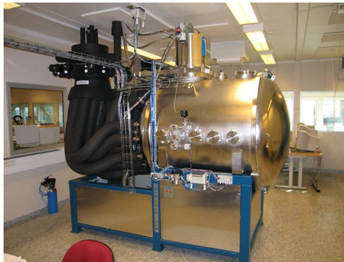
Figure 13: Image of one of Beyond Gravity's Thermal Vacuum Cycling chambers. This specific one has working area for test specimen: 600mm x 600mm x 600mm. Process pressure: 0.1 mPa. Pumping capacity at 1 mPa: 6000 l/s. Temperature range: -165°C - 180°C. [26]
