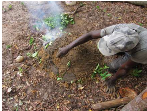
Figure 15: The pile covered in mud, set on fire from the end where the smoke emerges.
