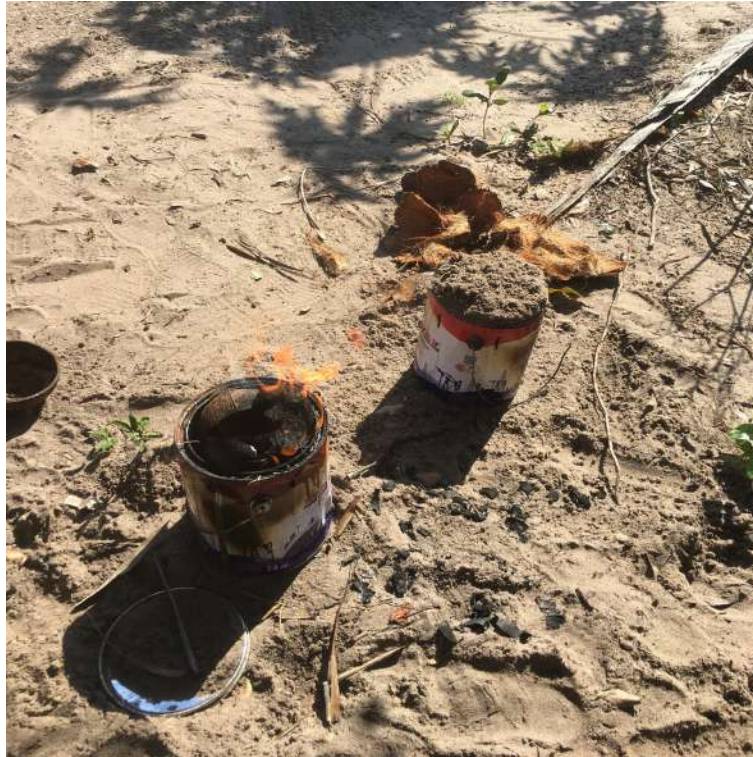
Figure 17: A metal kiln burning, and one covered with sand.
