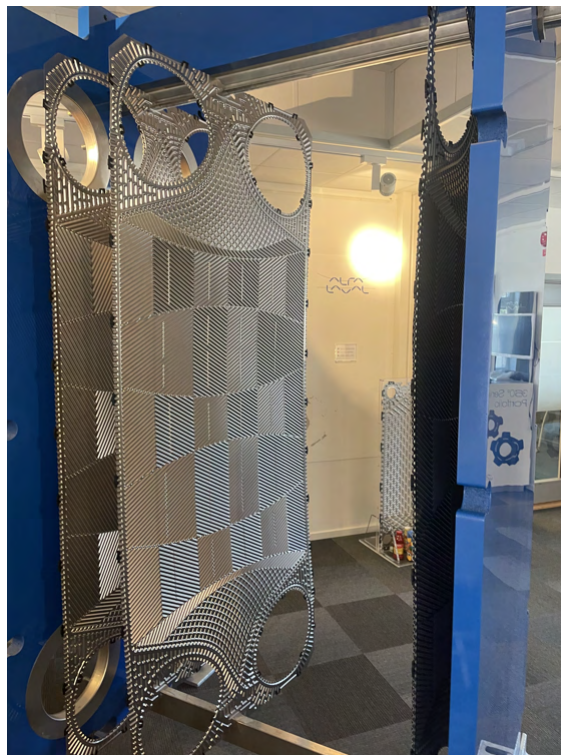
Figure 1.1: Partial Assemble Large Heat Exchanger, Showing Pressed Heat Exchanger Plate
