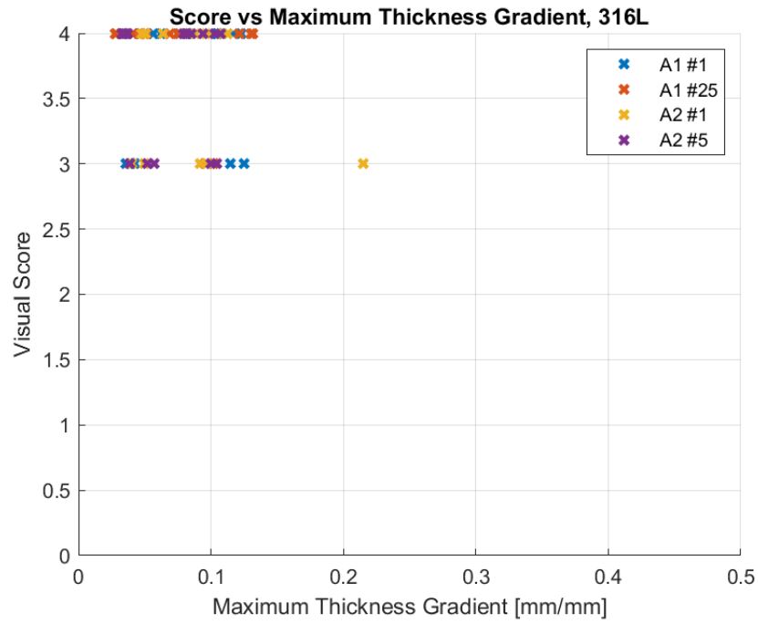
Figure 4.12: Relationship Between Maximum Thickness Gradient and Formability Score, 316L
