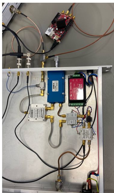
Figure 3.11: The new phase-modulator setup. The new PA2731 along with the logic controller can be seen at the end of the transmission (top side). Note that the trigger-input for the controller is missing in this image.
