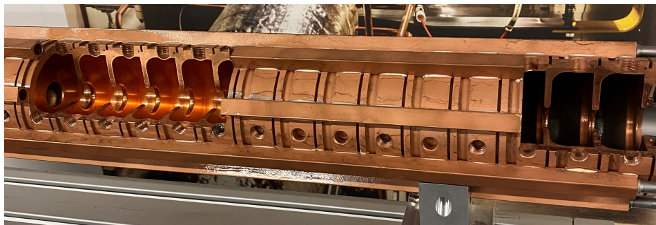
Figure 2.3: Cross-section of an S-band accelerating structure.
