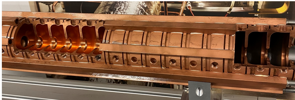
Figure 2.3: Cross-section of an S-band accelerating structure.
