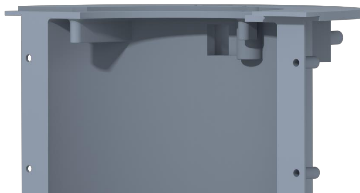
Figure 5.5. Redesign of screw towers for manufacturing purposes.
