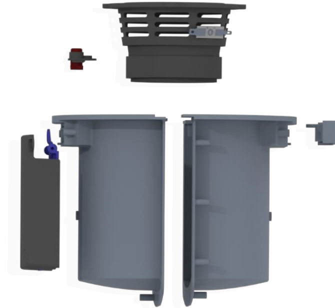
Figure 5.12. Exploded view of the smaller speaker.
