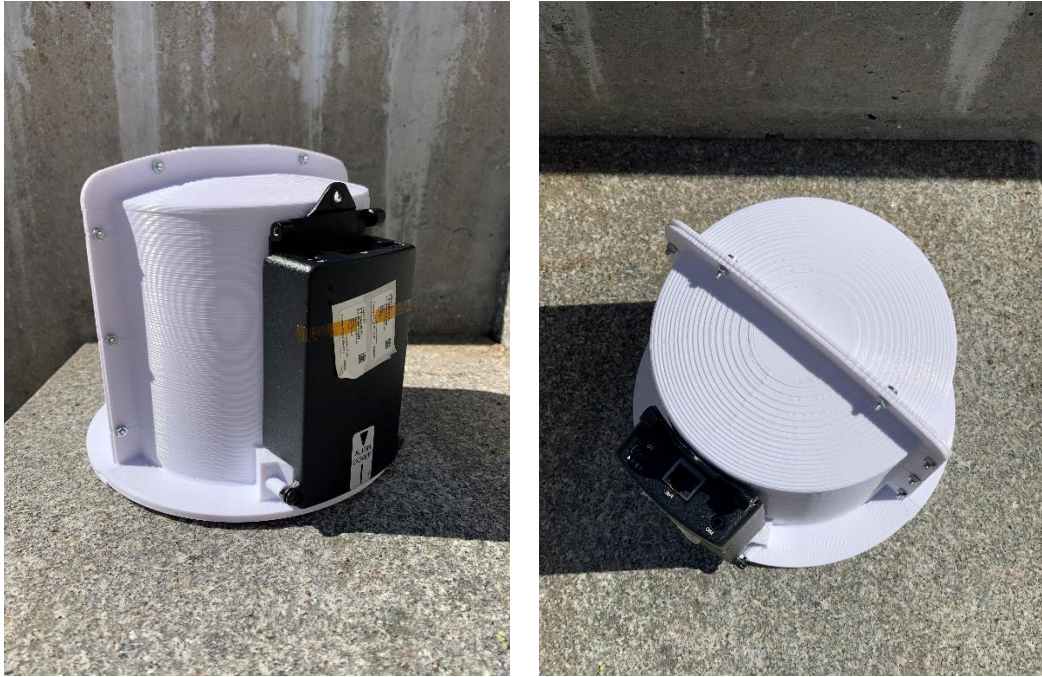
Figure 4.28. The mounted PCB-box on the smaller redesign and the redesign from above.
