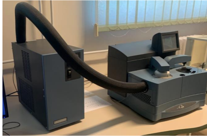
Figure 2.10 Differential scanning calorimetry equipment used for testing
