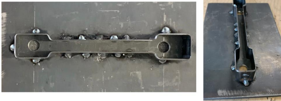
Figure 2.7 Final customized punching tool design
