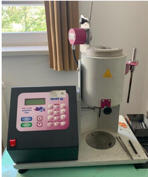
Figure 2.5 MFI equipment used for testing
