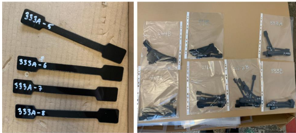
Figure 2.8 Tensile test specimens created with the punching tool
