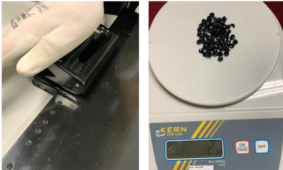
Figure 2.4 Procedure of collecting materials for MFI test
