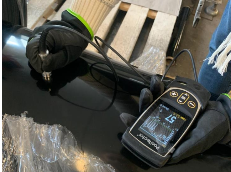
Figure 2.2 Shore D hardness testing with a durometer
