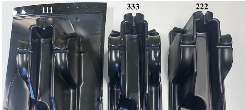
Figure 4.11 Appearance of tested material after thermoforming, illustrating finished products
