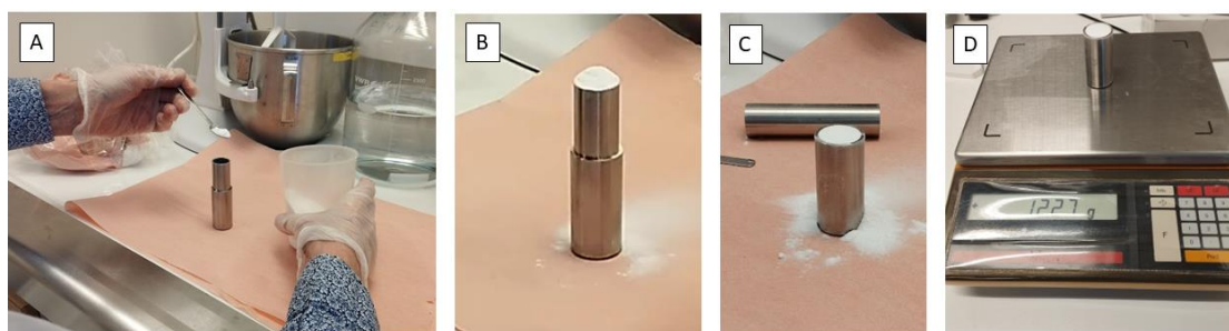
Figure 5 Poured bulk density process. A: Pouring of the powder mixture. B: Filled density test cylinder (20 ml). C: Scraped density test cylinder (20 ml). D: Weighted density test cylinder (20 ml).
