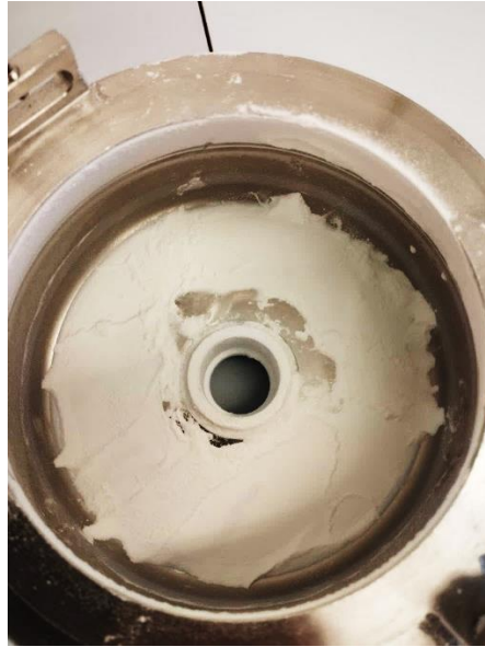
Figure 35 High shear mixer (Diosna® mixer PI-6) picture taken after the production of formulation 3. It can be seen high amounts of powder mixture impacted on the bottom of the mixer vessel, this amount was discarded.
