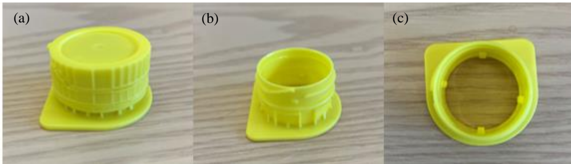
Figure 17 HeliCap™ 26 Pro (a) with lid (b) with the lid removed and (c) showing the knobs used for attaching to the fixture.
