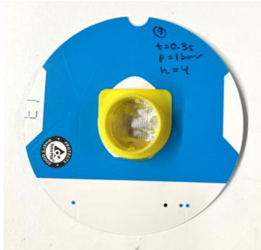
Figure 13 Specimen with cap applied at the PLH.
