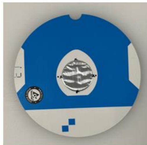
Figure 10 Specimen with four marks around the PLH showing where the defects are created.
