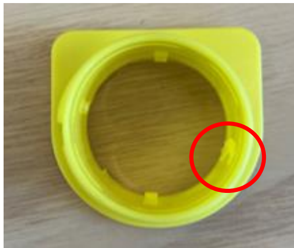
Figure 29 HeliCap™ 26 Pro with broken knobs from using the first edition of cap detachment fixtures.
