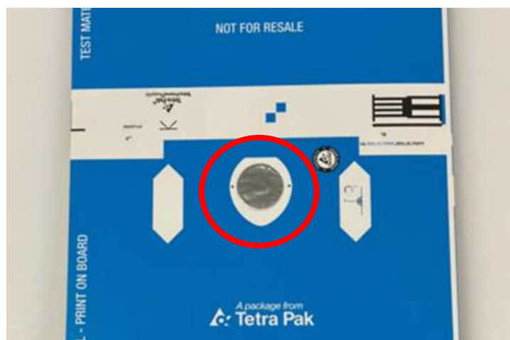
Figure 4 Packaging material with PLH (circled) where the cap is to be attached during package production.
