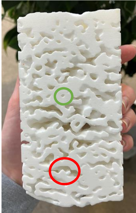
Figure 3 3D printed model of cross-section of a paperboard with clay coat layer on top showing both the cavities within the fibres (green circle) and the pores (red circle). The model is not to scale.
