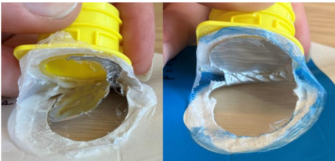
Figure 45 Delamination between décor layer and clay-coat for large degree ES.
