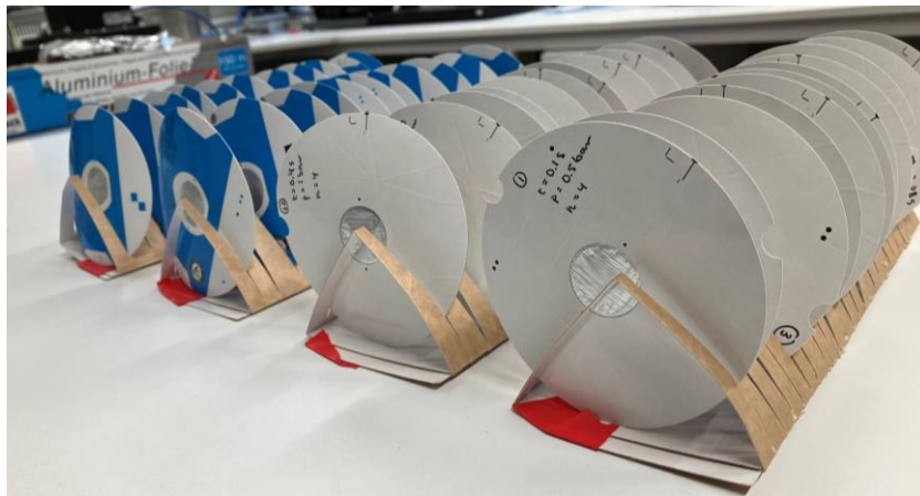
Figure 16 Specimens placed in climate-controlled environment for two weeks to acclimate the paperboard.
