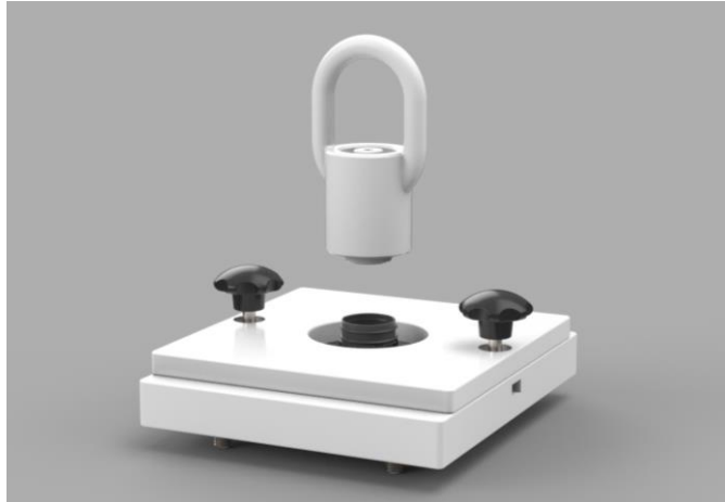
Figure 28 Visual of the 3D-printed fixtures created to measure cap detachment force.
