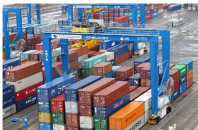
RTG, Rubber-Tired Gantry Crane (Konecranes, No date)
