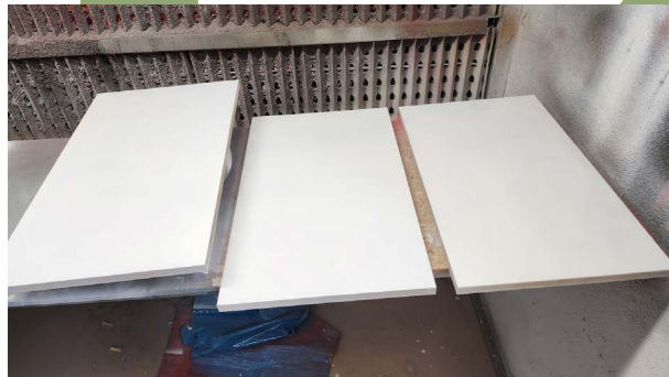
I painted the 20mm MDF shelves white so that they would match the rest of the hutch.
