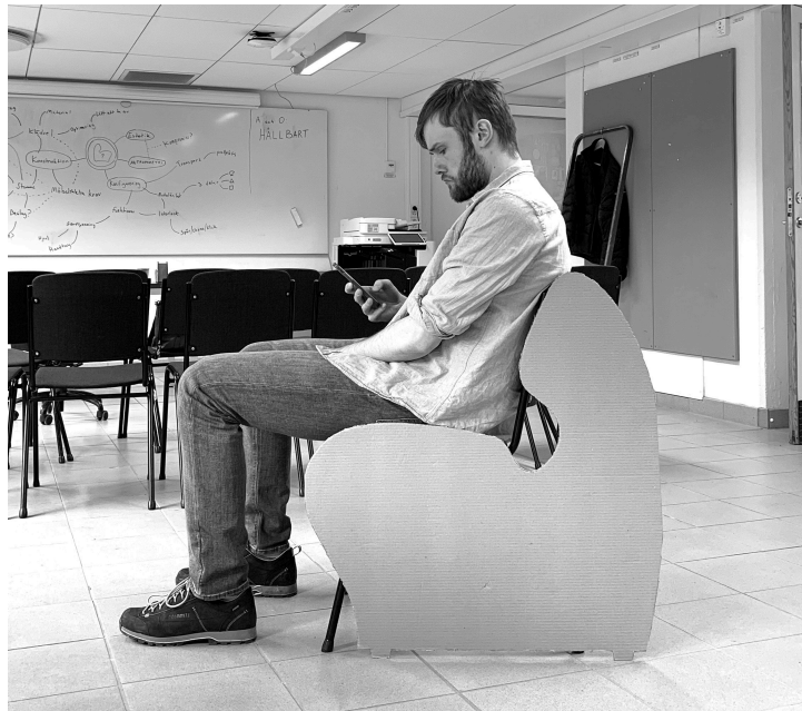
Figure 9.9 Cardboard Cutout Size Test.
