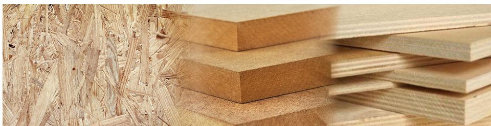
Figure 8.1 From left to right: particle board, MDF and plywood.
