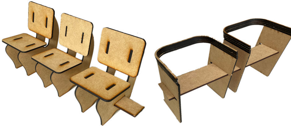
Figure 9.3 Models cut from MDF by a laser cutter, from Sprint 1.
