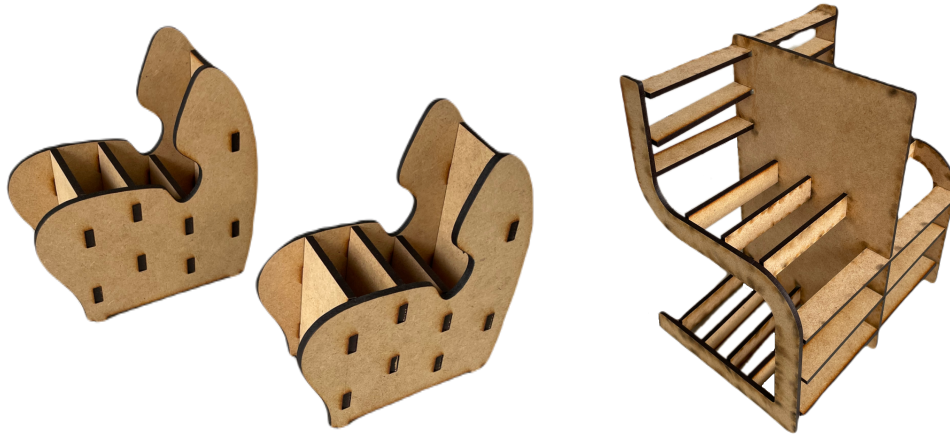
Figure 9.6 Models cut from MDF by a laser cutter, from sprint 2.
