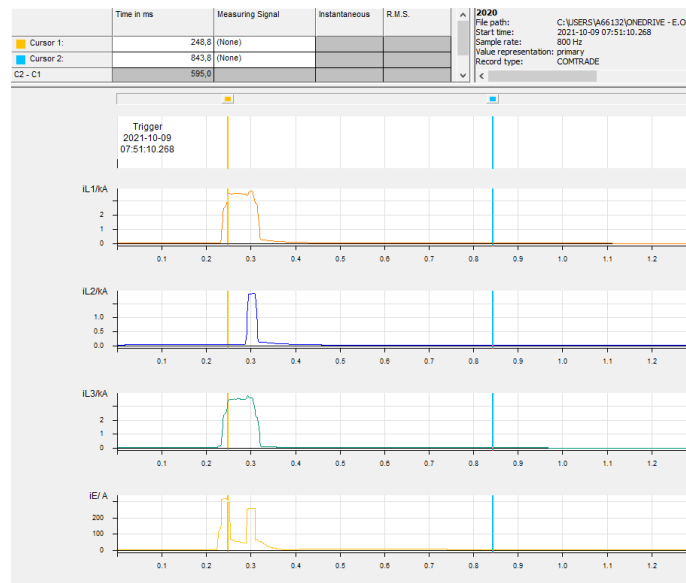
Figure 5.19: Phase currents during 9/10-21 fault recorded at bay "F3" in STM
