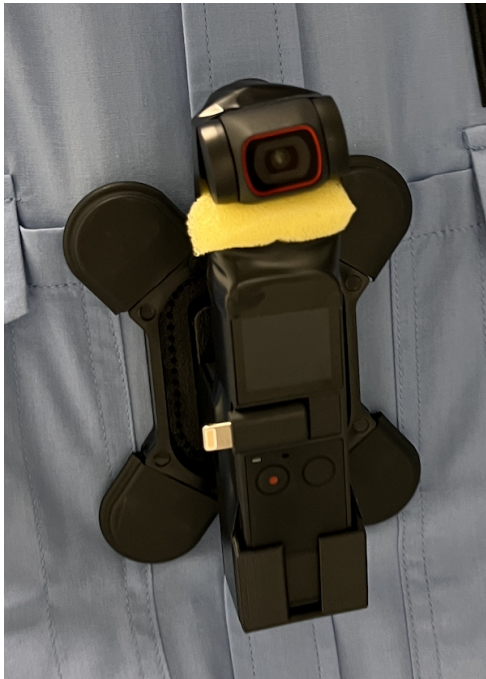
Figure 20: DJI Pocket 2 with a disabled gimbal.
