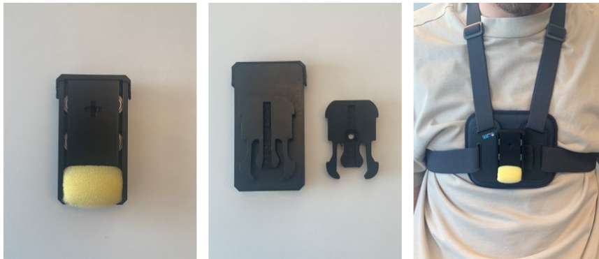
Figure 8: 3D-printed fixture and harness solution
