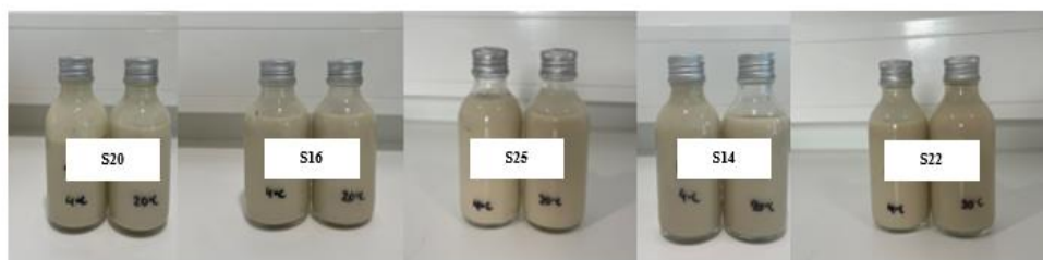
Figure 8 The samples from the trial with 14% total protein after 2 weeks of storage at 4°C and 20°C. For sample codes, see Table 4.
