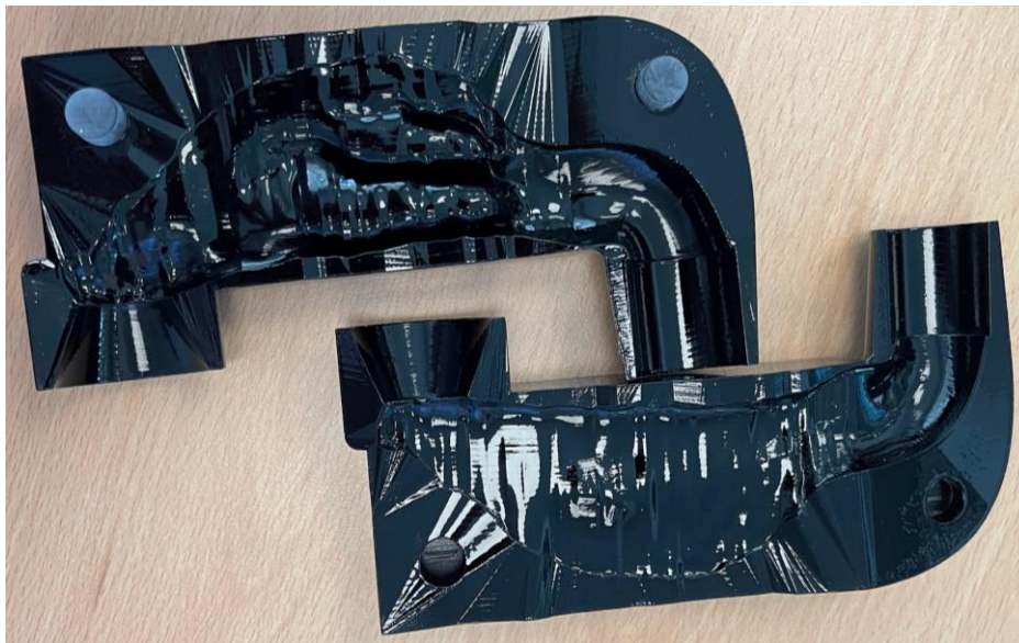
Figure 2.3. The 3D-printed nasal cavity model replicating the human nasal cavity. The two halves together form one of the two nasal cavities.
