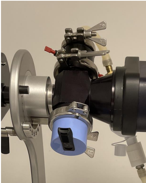
Figure 2.2. The setup for the SprayTec analysis with the ICOone nozzle and ICOone Nasal device attached.
