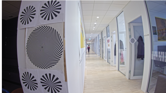
FIGURE 8.28: A person at a distance of 18m away from the camera. The image is taken by the M3088 prototype 2. Close up can be seen in 8.31.
