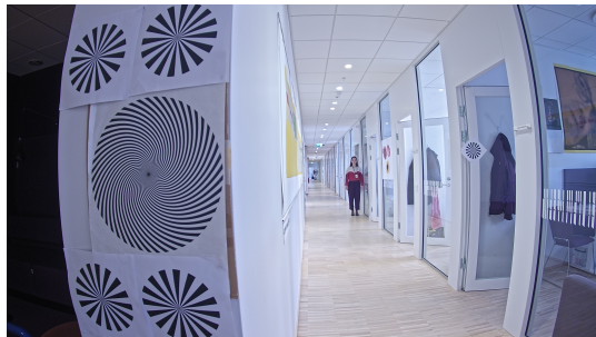
FIGURE 8.29: A person at a distance of 6m away from the camera. The image is taken by the M3088 prototype 2. Close up can be seen in 8.32.
