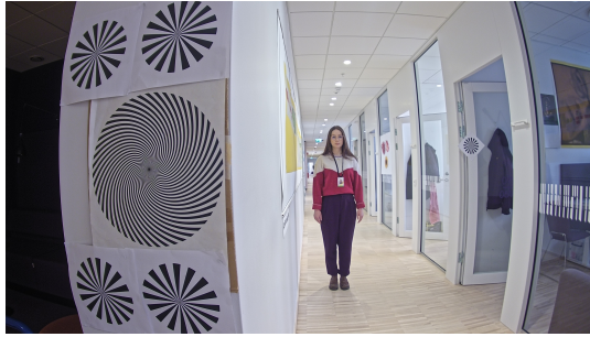
FIGURE 8.30: A person at a distance of 3m away from the camera. The image is taken by the M3088 prototype 2. Close up can be seen in 8.33.
