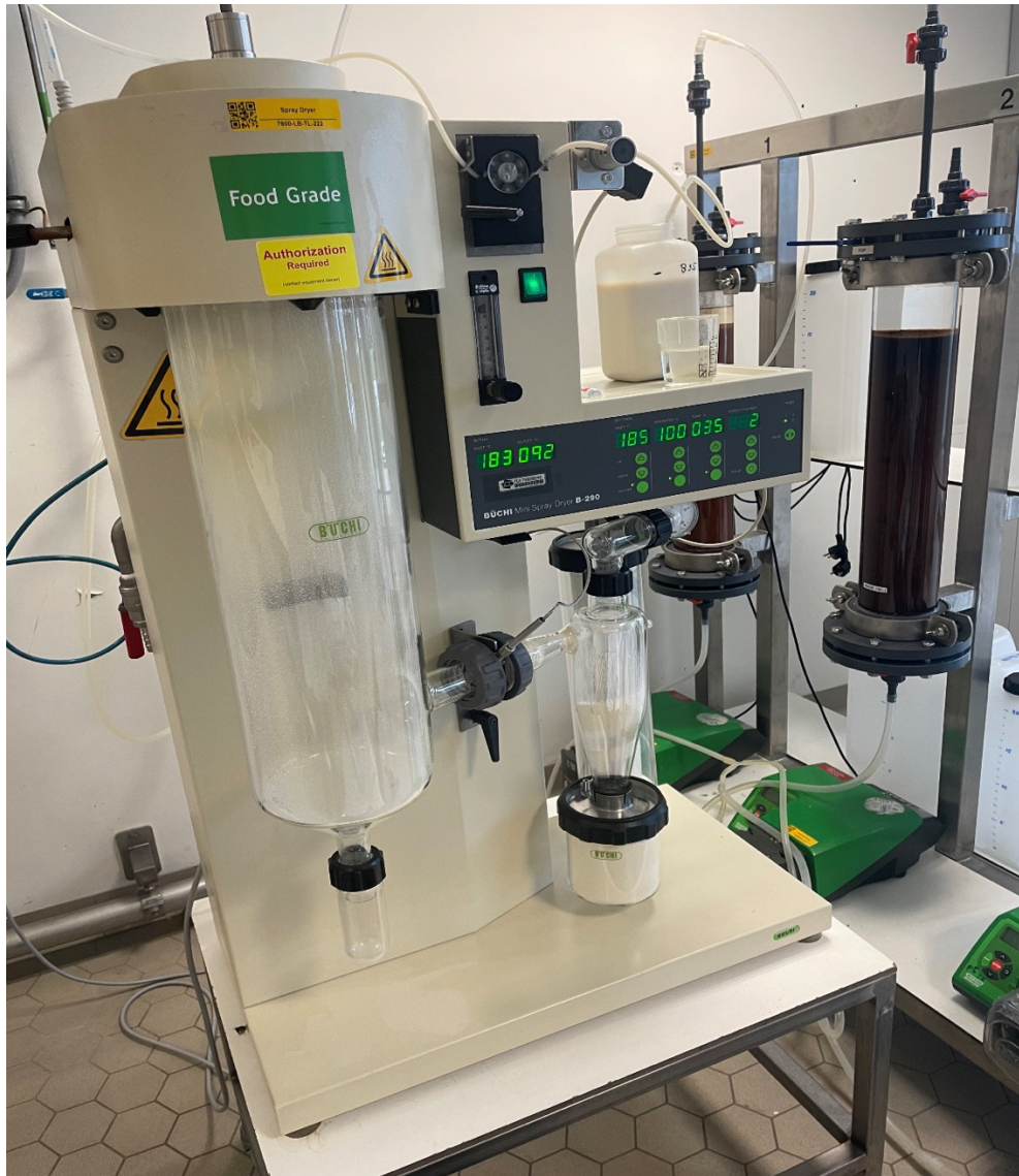
APPENDIX E: Buschi mini spray dryer. Equipment used for the spray drying of the fermented pea protein
