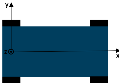
Figure 10: The orientation of the local coordinate system for the ego vehicle with the origin in the middle of the rear axis.
