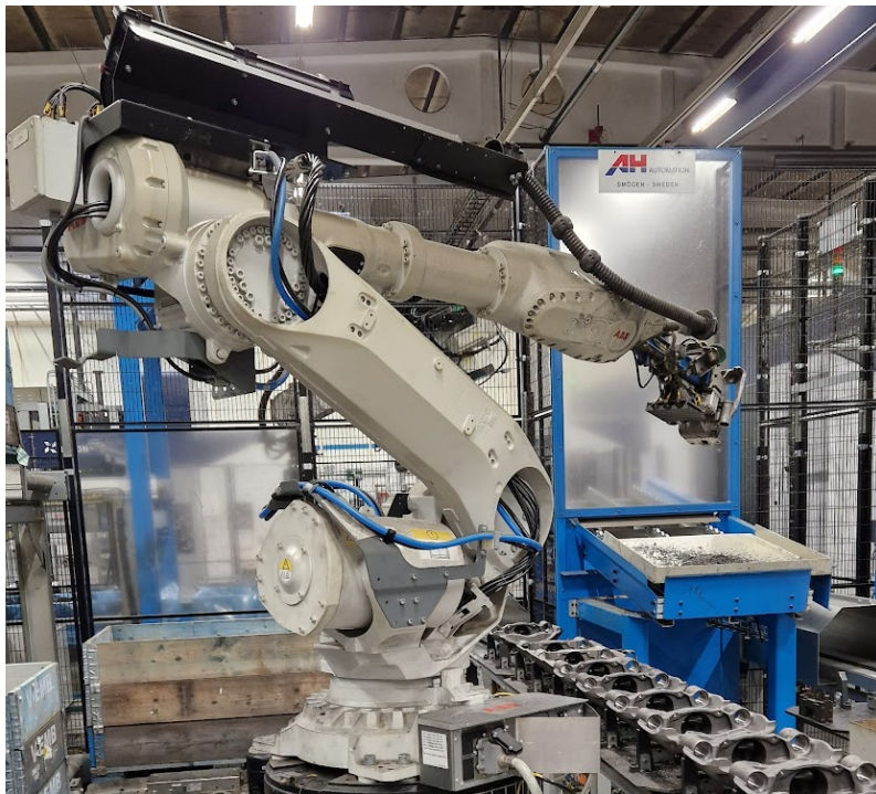
Figure 3.10: Central robotic arm in the LiCON cell performing the "shaking motion".
