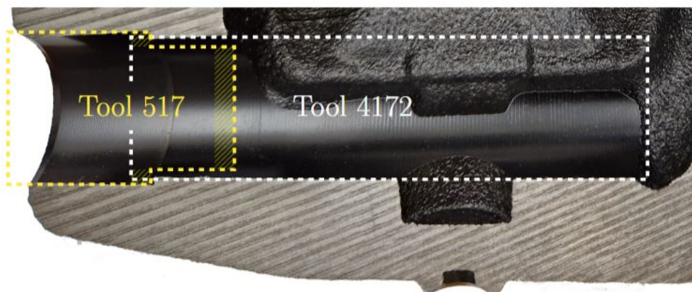
Figure 7.9: Tool utilization in machining and feed reduction region in machining of feature ②.
