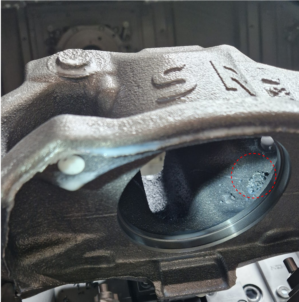
Figure 6.7: Internally remaining chips prior to flushing when ending machining with feature ④ (Drilling and reaming).
