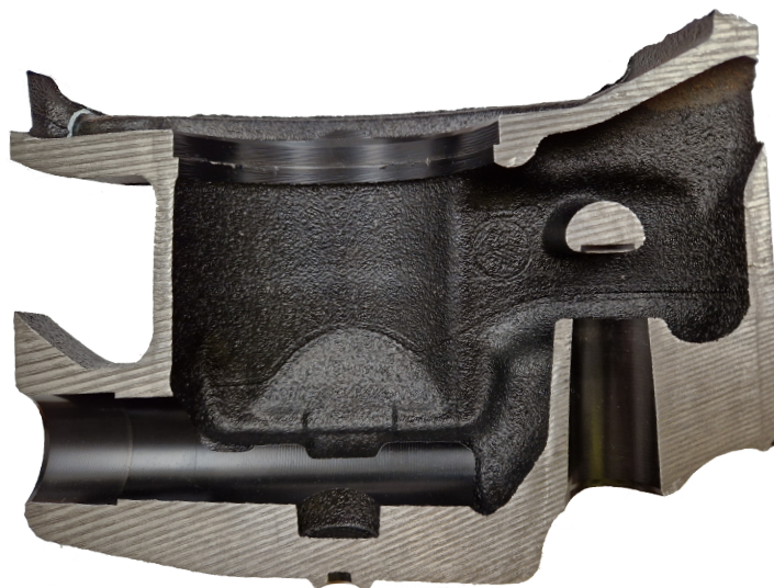
Figure 3.2: Cross section of caliper housing (SAF model in the right hand orientation).
