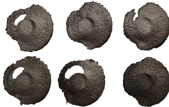
Figure 5.12: Disc burrs from the machining operations of the 19 inch brake caliper model.
