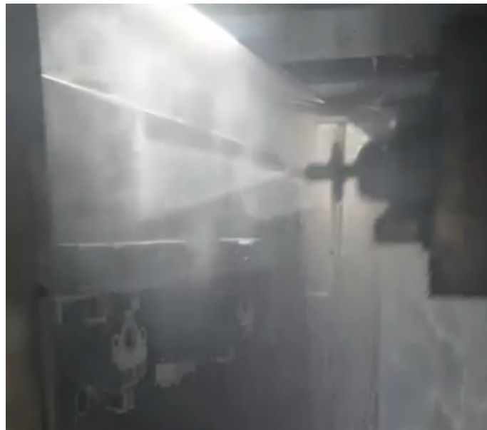
Figure 6.6: Spray pattern of internally cooled tool (which could be used for flushing).
