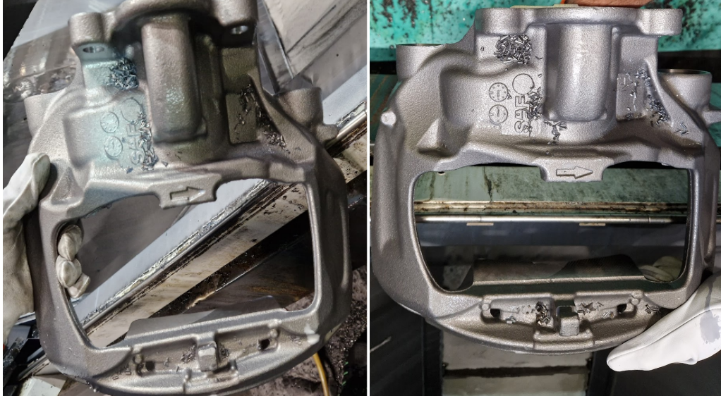
Figure 5.17: Effectiveness of flushing operation on machined calipers (Left: no flushing, right: flushed).
