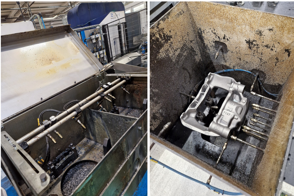
Figure 3.9: Compressed air fixtures (CAF) for chip removal; generic CAF (Left), specialized CAF (Right).
