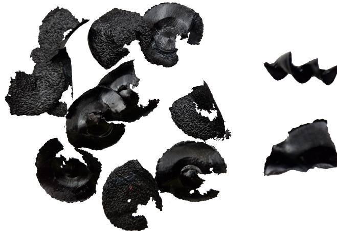
Figure 3.13: Coated chips found in testing after coating operations have been completed at the EDC facility.
