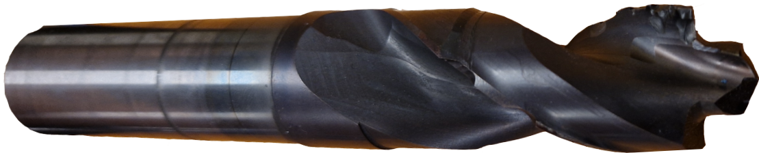
Figure 7.12: Double fluted twist drill dedicated for machining of feature ④; detail of chipped cutting edge which caused tool failure.
