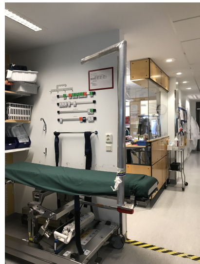
Figure 3. Supporting arm physical prototype attached to an operating table at BUS.
