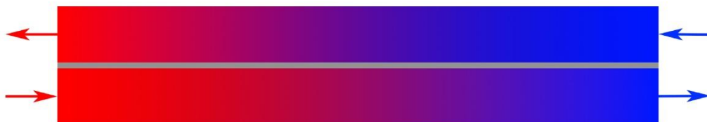
Figure 3: A visualization of a counter flow heat exchanger. The top half feeds in a cold fluid and the bottom half feeds in warm. The gray area in between is a thin metal plate conducting heat between the fluids.
