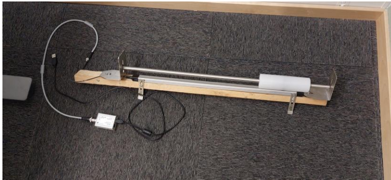
Figure 13 Setup for the angle impact test. The MPA sensor is mounted on the wooden plank, and the grey I/O link is placed in front of the plank.
