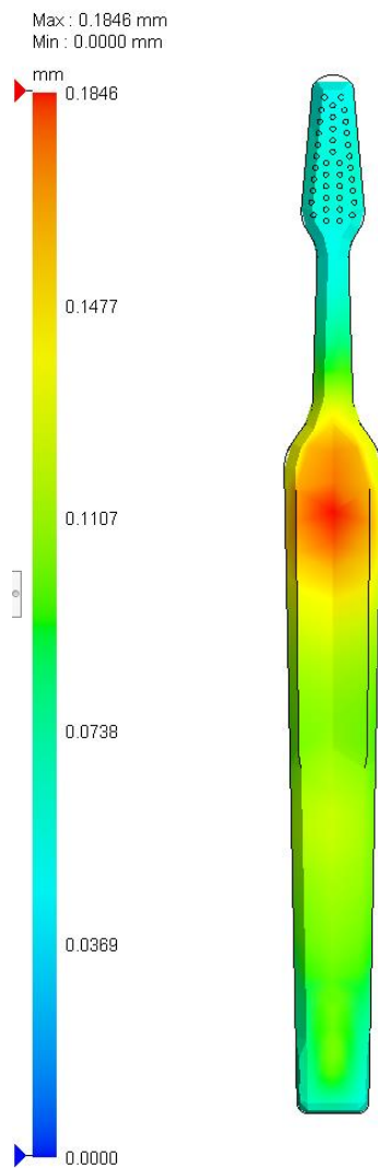
Figure 3.7 The red area is cooling down slower than other areas in the toothbrush.
