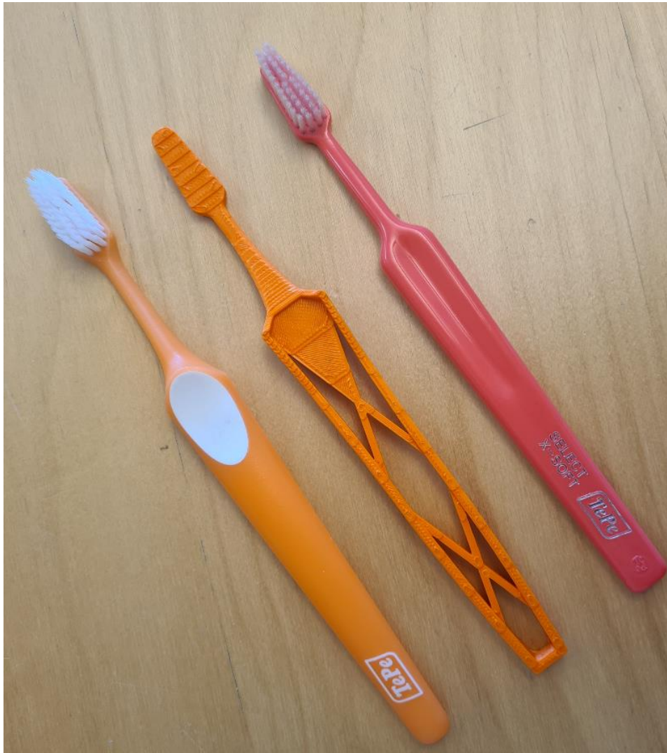
Figure 4.28. Prototype made by FDM.
