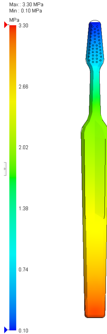
Figure 3.5 Color-coding of toothbrush based on the pressure at end-of-fill.
