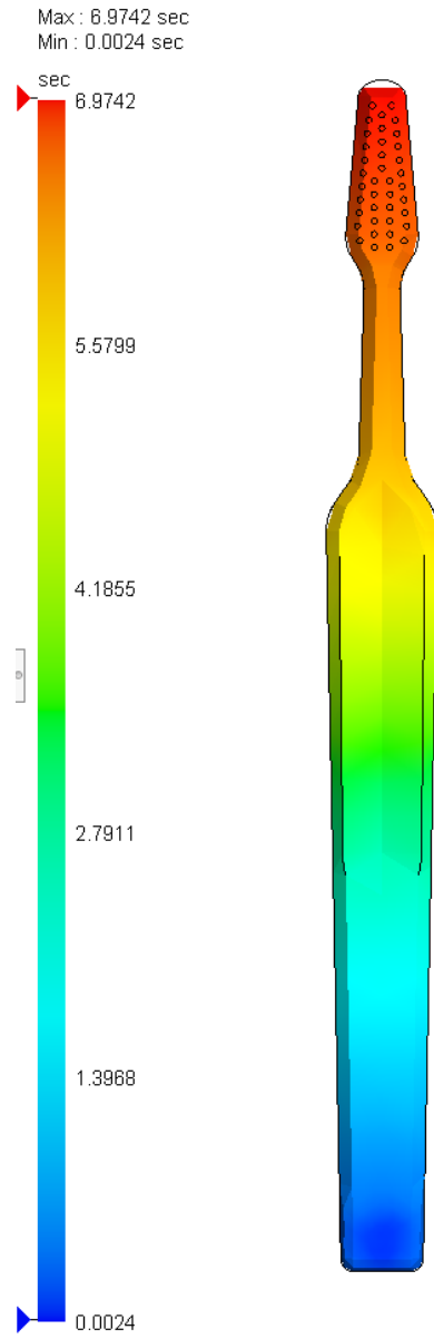
Figure 3.3 The result of running a mold flow analysis of the reference toothbrush.
