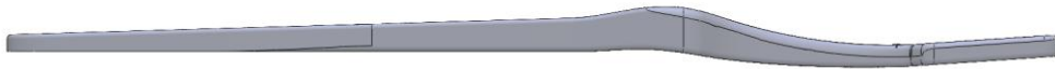
Figure 4.50. Sideview of the final concept, with 3 mm of thickness at the bottom.
