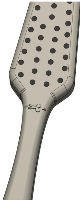
Figure 4.52. Symbol to make recycling easier for the customer.
