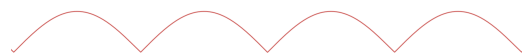
Figure 3.10: An absolute valued sine wave. Showing how one can get sharper valleys and doubled the number of smooth peaks.
