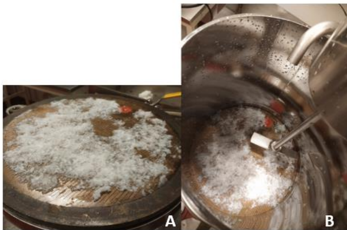
Figure 40 (A) Reject material from repulped uncoated material left after passing through 40µm screen (B) The sommerville defibrillator tank.
