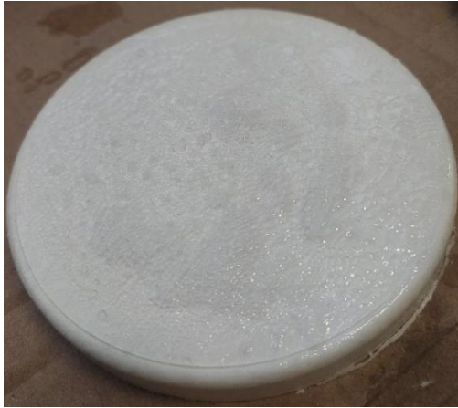
Figure 15 Crystallization after drying in V4.
