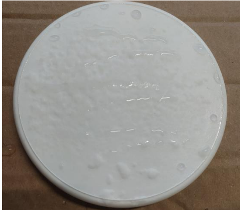
Figure 12 Spray coating showing good barrier property at the corners only.
