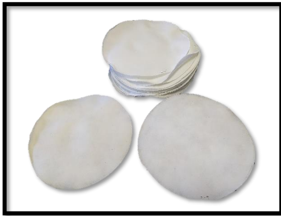
Figure 28 Handsheet of 20 min defibrillated accept material.
