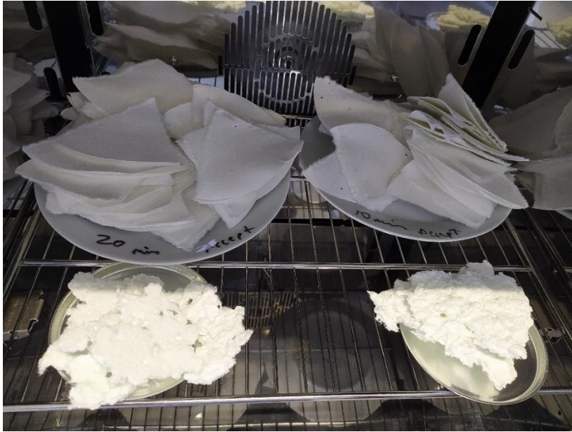
Figure 48 Drying of handsheets and reject material for yield calculation.
