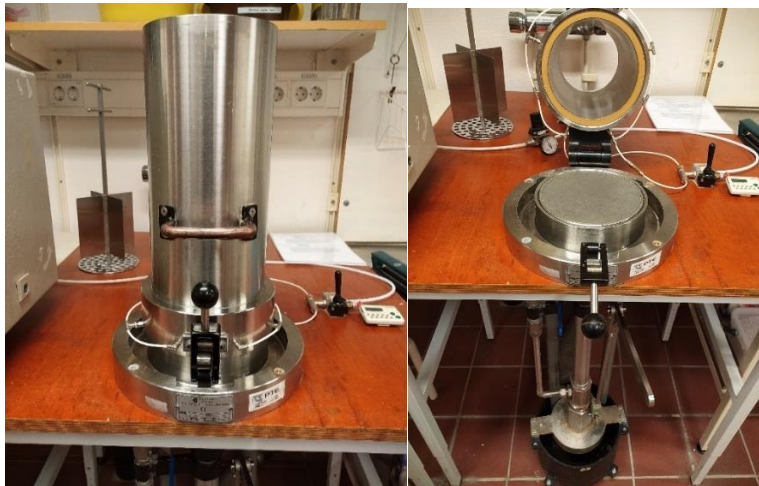
Figure 42 The handsheet former (left) and the mesh used to form the handsheets (right)
