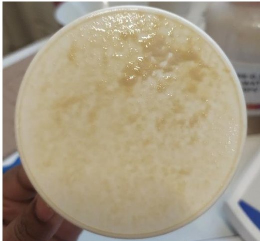
Figure 13 Rough texture of the sample coated by V3.
