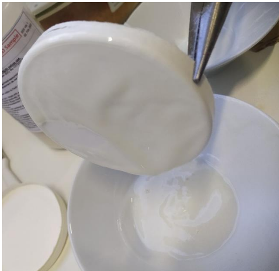
Figure 33 The unevenness in dip coating varnish 9.
