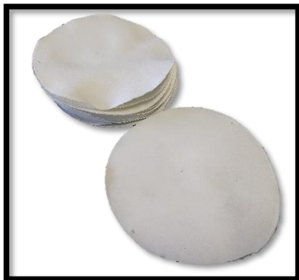
Figure 29 Handsheet of 20 min defibrillated accept material for coated lids.
