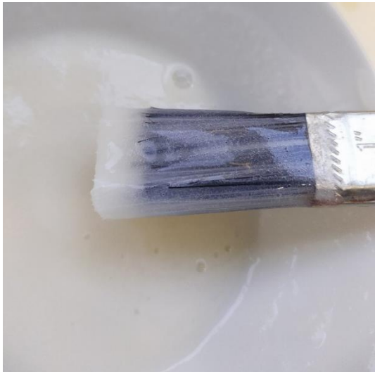
Figure 32 Highly viscous varnish with small air bubbles.
