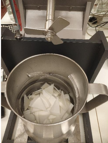
Figure 37 Samples and water inside the disintegrator for repulping
