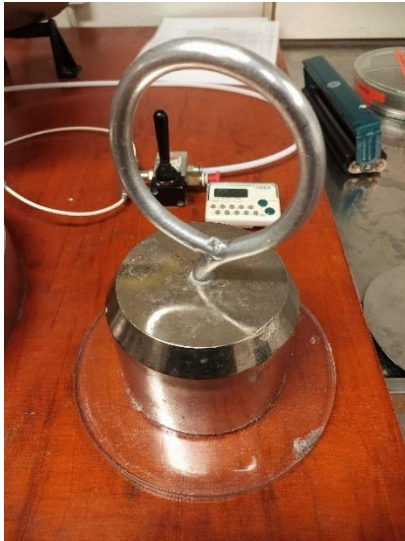
Figure 43 The gusk weight used to press the handsheet with the blotting paper to remove the excess water.
