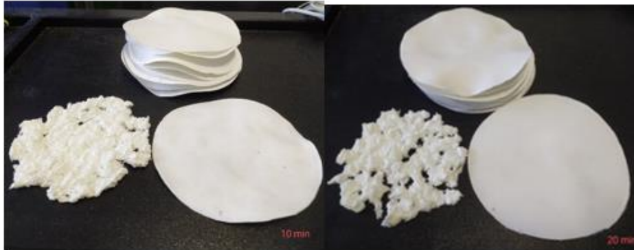
Figure 46 Handsheets from the coated (varnish 6) lid's repulped material Handsheet of 10min (left) and 20min (right) defibrillated accept material.
