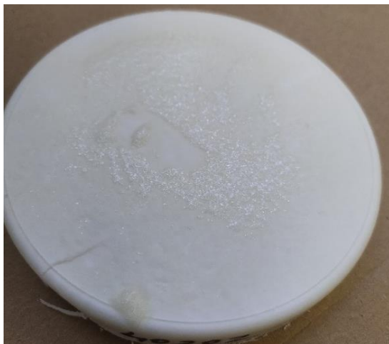
Figure 14 The wafer formation observed in V9 after drying for 10 min due to over coat weight.
