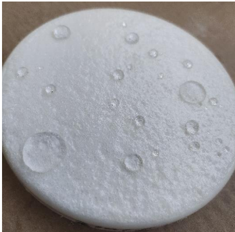
Figure 16 Bubbly texture with excellent water barrier property after drying in V6.
