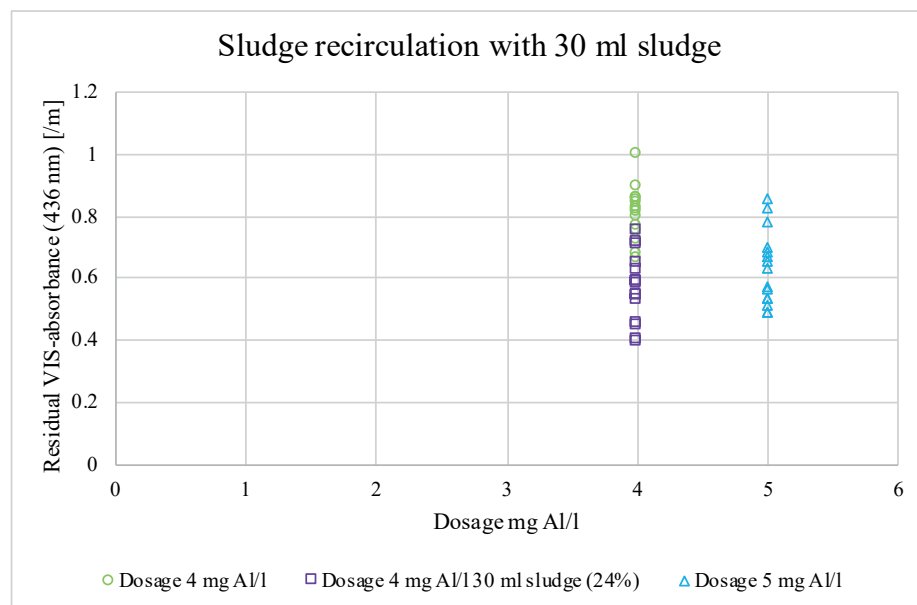
Figure 23: Residual VIS-absorbance at 436 nm showing effect of 30 ml sludge at 4 mg Al/l (purple squares) compared to 4 and 5 mg Al/l with no added sludge (green rings and turquoise triangles, respectively). The sludge was produced on the 3 rd of April.
