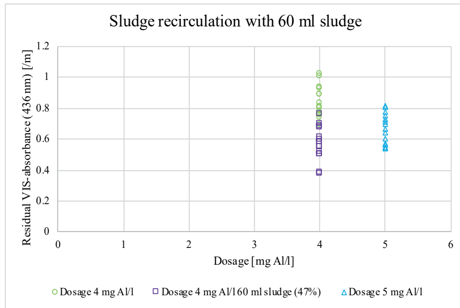
Figure 22: Residual VIS-absorbance at 436 nm showing effect of 60 ml sludge at 4 mg Al/l (purple squares) compared to 4 and 5 mg Al/l with no added sludge (green rings and turquoise triangles, respectively). The sludge was produced on the 3 rd of April.
