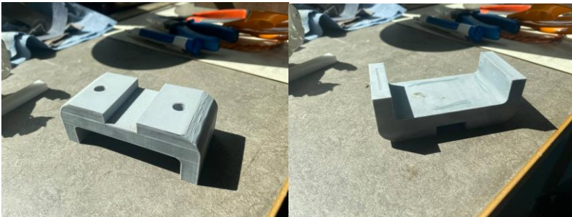
Figure 55 3D printed ferrite cooler
