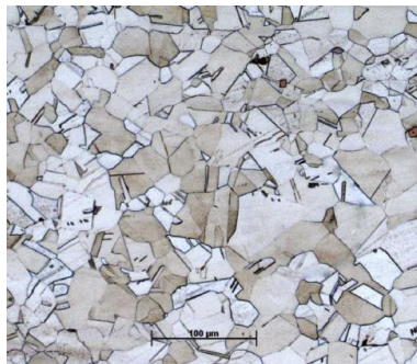
Figure 14 Metallographic photo of medium manganese austenitic steel ( Shirong Ge, 2017 )
