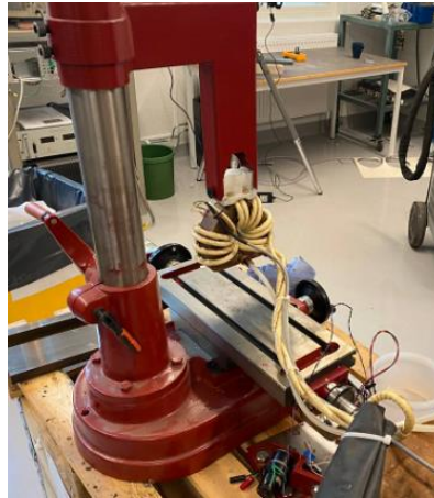
Figure 20 Pencil machine for the testing of the coils
