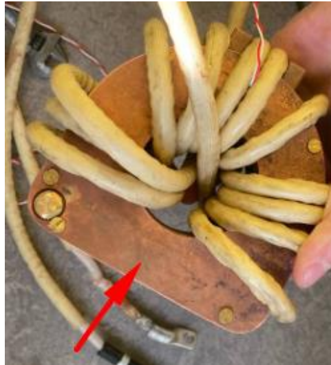
Figure 46 Point of the highest temperatures in the heating unit
