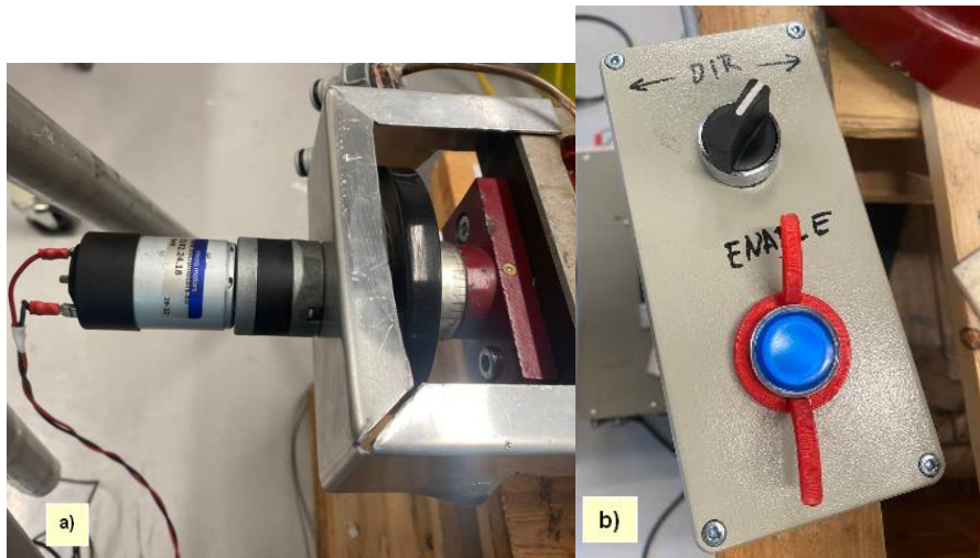
Figure 21 a) DC motor for movement in y direction b) control box
