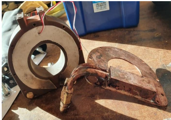
Figure 48 Cooling added to the lid
