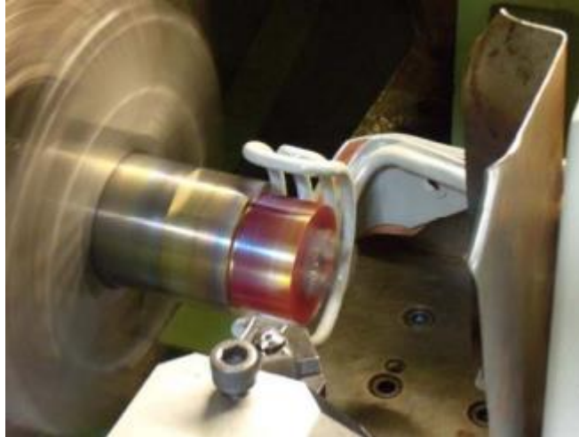
Figure 5 Semicircular induction coil (Baili M, 2011)
