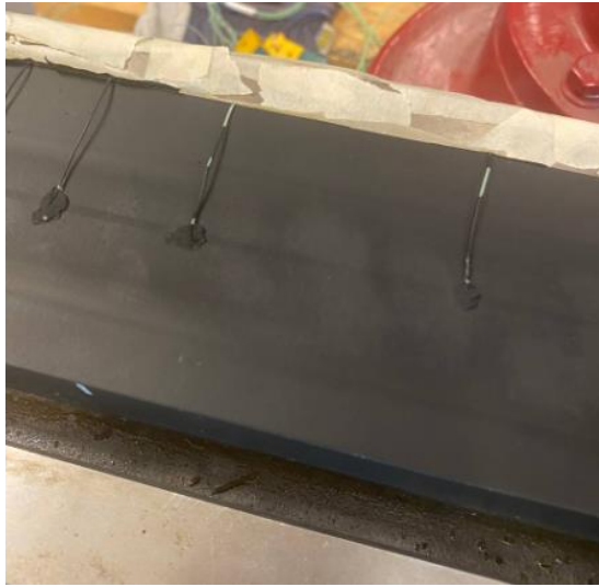
Figure 27 Prepared workpiece with glued thermocouples
