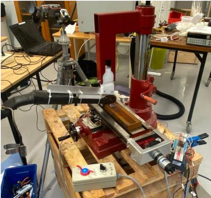
Figure 30 Fully assembled testing equipment (Low frequency heating unit)
