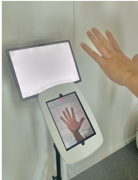
Figure 3.1: The intended setup for the contactless palm print recognition system.
