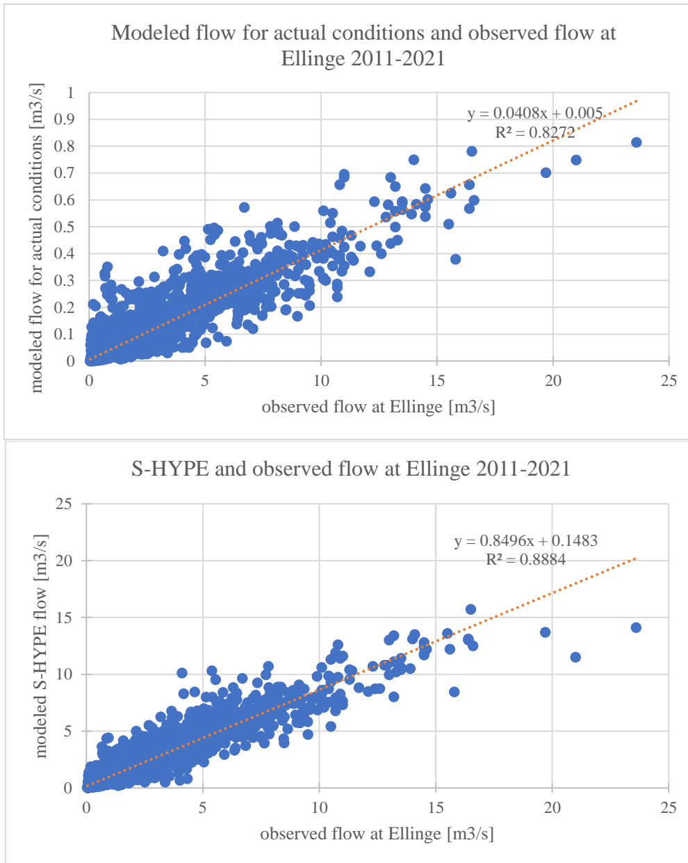
Figure 13. Correlation between modeled HYPE flow and observed flow at Ellinge 2011-2021 (upper figure) and correlation between S-HYPE and observed flow at Ellinge for 2011-2021 (lower figure). Modeled flow on the Y-axis ranges from 0 – 1.3 m 3 /s for the upper figure and from 0 – 25 m 3 /s for the lower figure.
