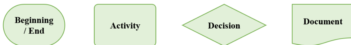
Figure 17: Symbols commonly used for different activities in a process map (Ornat & Moorefield, 2019)
