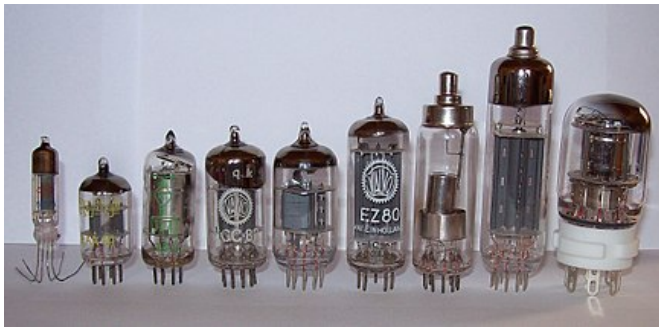
Figure 2.1: Vacuum tubes, the predecessor to transistors [4]
