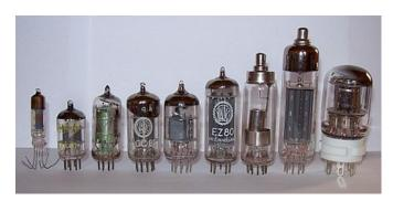
**Figure 2.1:** Vacuum tubes, the predecessor to transistors [4]
