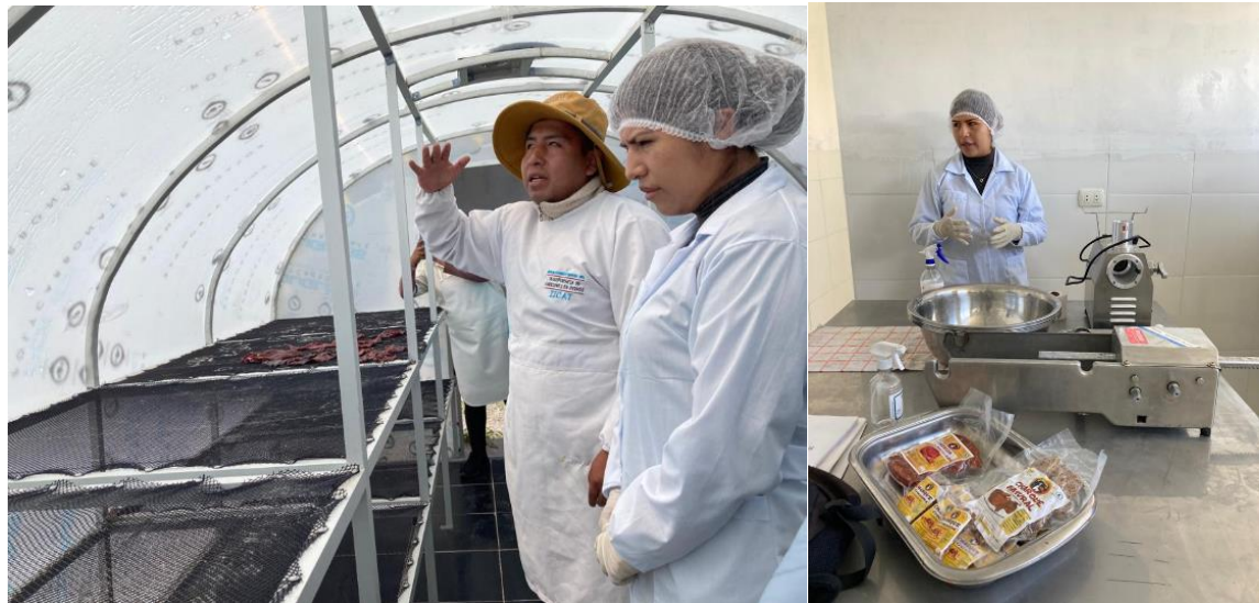
Figure 6-1. Facilities of llama meat producers. Left: solar dehydrator. Right: llama meat product and electric meat tenderizer
