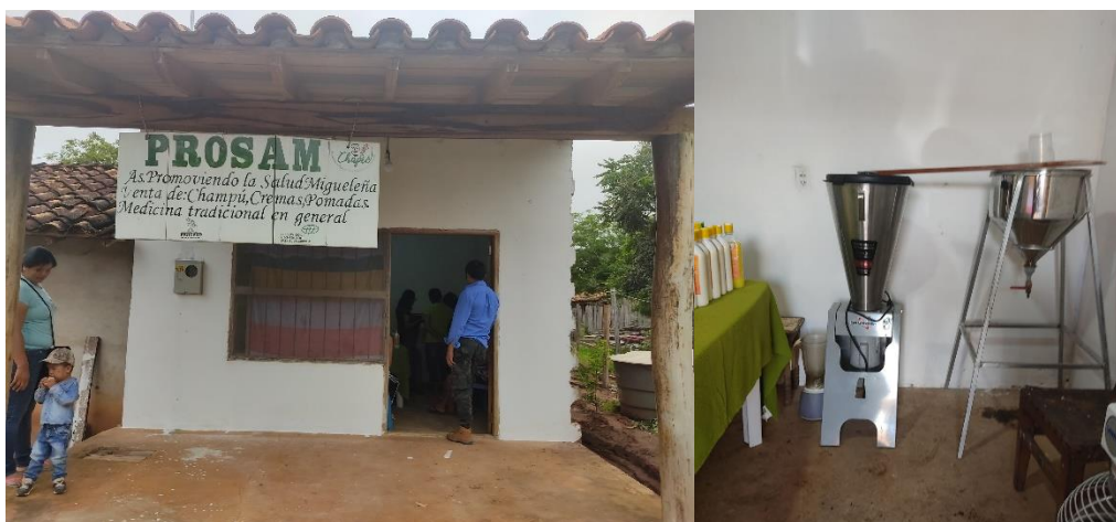
Figure 6-5. Left: organization facilities. Right: Electric mixer and blender for shampoo production. Source: taken by the author
