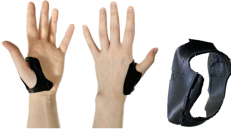
Figure 6.12 The resulting rigid hand part going around the thumb.
