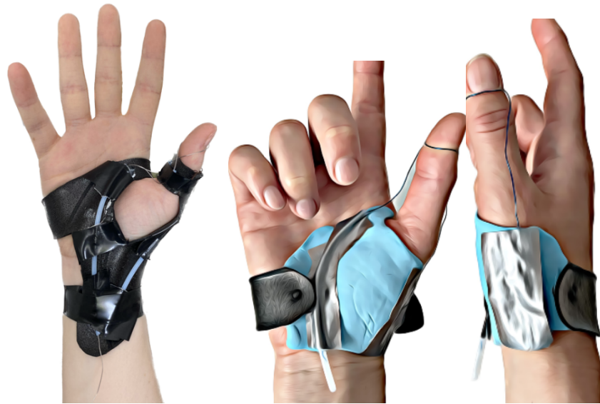
Figure 6.5 PVC prototype with plastic tubes and wire (left) and prototype in two component silicone (right).
