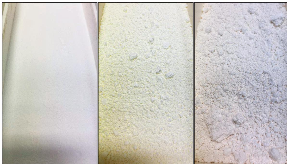
Figure 21: Original powder of Puralox to the left, CeZr in the middle and Y-zeolite to the right.
