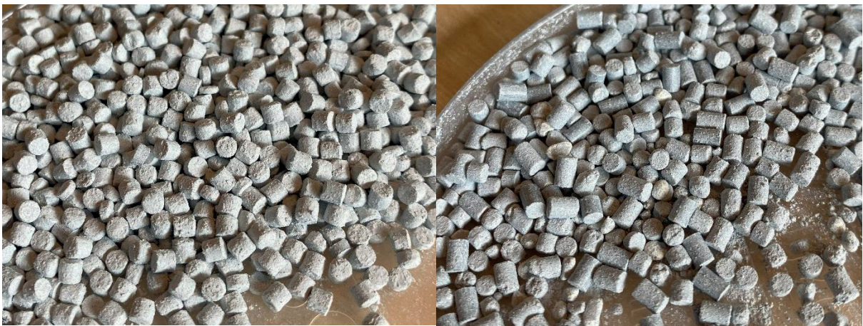
Figure 23: Tablets of original CeZr powder to the left and spray-dried CeZr powder to the right.
