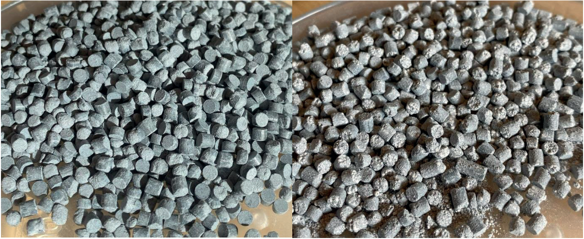
Figure 22: Tablets of Puralox powder to the left and spray-dried Y-zeolite to the right.
