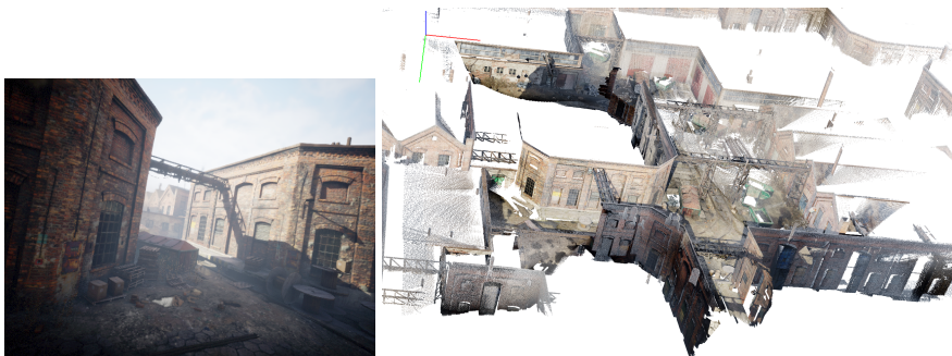
Figure 8: The Abandoned factory sequence from TartainAir. Left: One frame illustrating the synthetic RGB image. All pixel depth values of this frame can be extracted from its corresponding depth map. Right: Abandoned factory ground truth in its entirety, after converting depth maps to a unified point cloud. Sparse segments imply only a few frames have captured those parts, with little overlapping areas between images.
