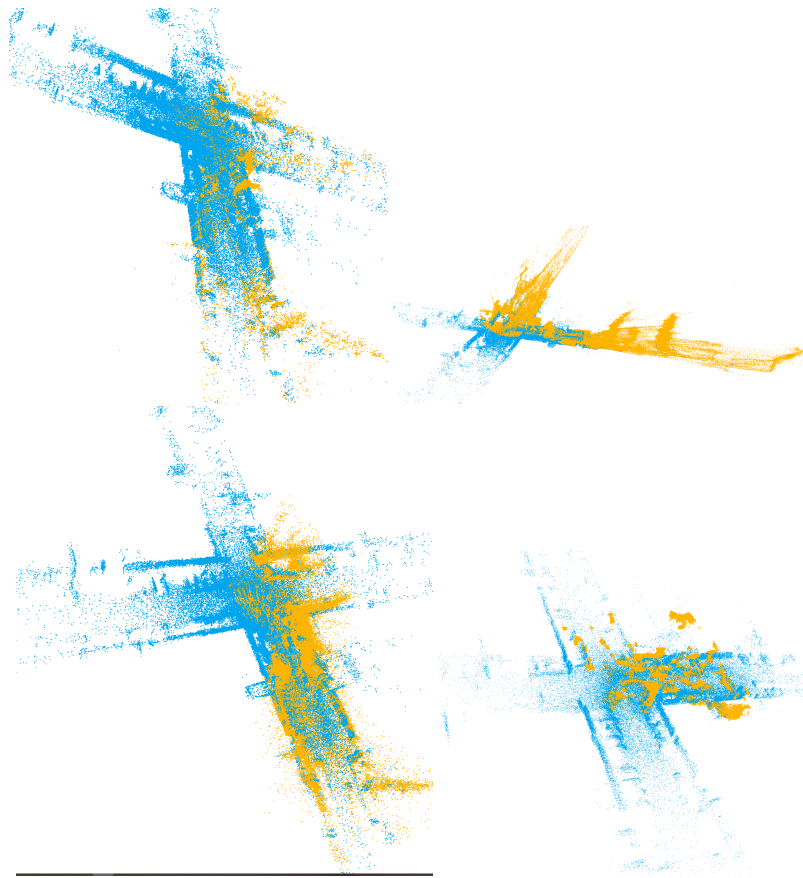
Figure 29: KITTI sequence; Aligning the estimated point clouds ( orange ) to the ground truth ( blue ) via ICP Registration. Top Left: COLMAP Sparse. Top Right: COLMAP Dense. Bottom Left: DROID-SLAM. Bottom Right: NeRF-SLAM.
