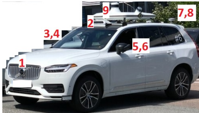
Figure 11: Image of the data-gathering car used to capture the images used in this thesis. The forward-facing fisheye and long-range cameras are highlighted with 1 and 2 respectively. 3, 4 and 5, 6 marks the positions of the short- and long-range fisheye cameras mounted on the side-view mirrors. 7, 8 shows the location of the GPS/GNSS receiver and IMU. Finally, 9 shows the position of the LiDAR.
