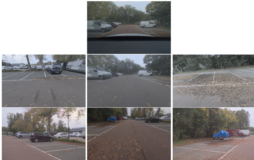
Figure 13: Rectified images from the second sequence, captured by all of the cameras. Top: Forward-facing long-range camera. Top row, left: Short-range fisheye camera mounted on the left side-view mirror. Top row, middle: Forward-facing short-range fisheye camera. Top row, right: Short-range fisheye camera mounted on the right side-view mirror. Bottom row, left: Long-range fisheye camera mounted on the left side-view mirror. Bottom row, middle: Rear bumper fisheye camera. Bottom row, right: Long-range fisheye camera mounted on the right side-view mirror.
